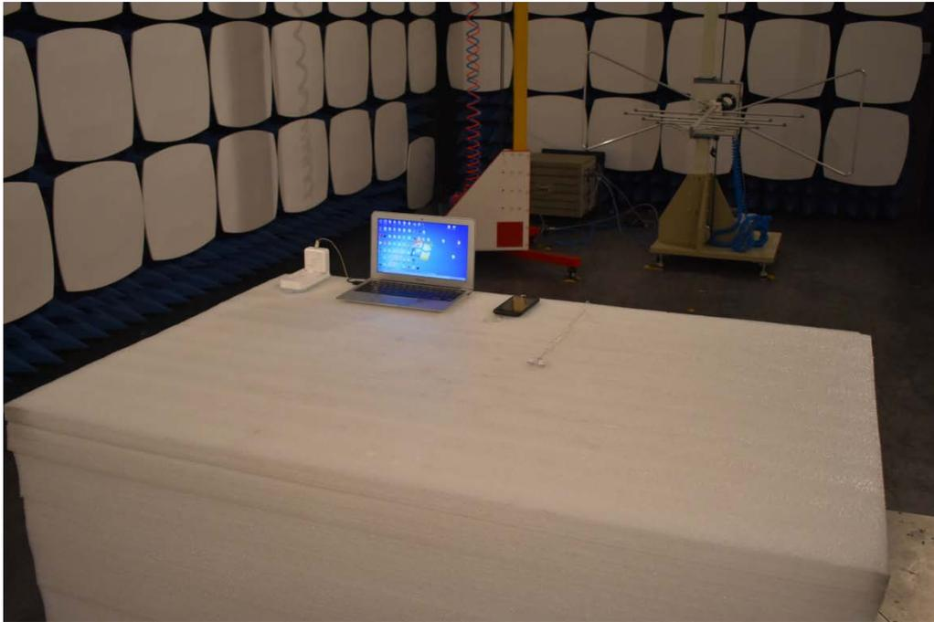
4. Radiated Field Strength Measurement(above 1GHz)
