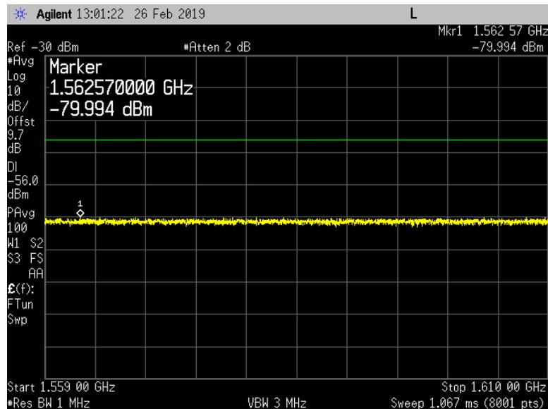
**Band 12 and Band 14 LTE10 Single Narrow Band IoT Upper Guard Band Carriers (80W/Port)**
