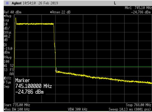
IoT Guard Band Carrier at Upper Placement
