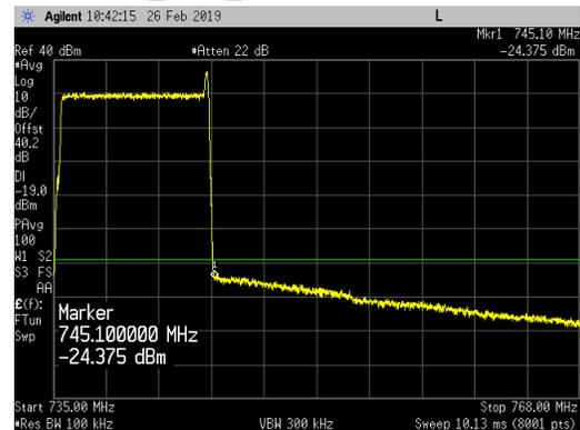
**Band 12 Single Narrow Band IoT Guard Band Carrier -Lower Band Edge Plots:**
