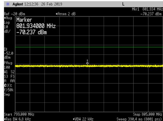
**Band 14 Single Narrow Band IoT Guard Band Carrier -Lower Band Edge Plots:**
