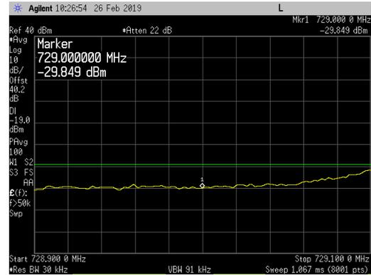
**Band 12 LTE10 at Top Ch (740MHz) 80W Single Narrow Band IoT Guard Band Carrier -Upper Band Edge Plots:**
