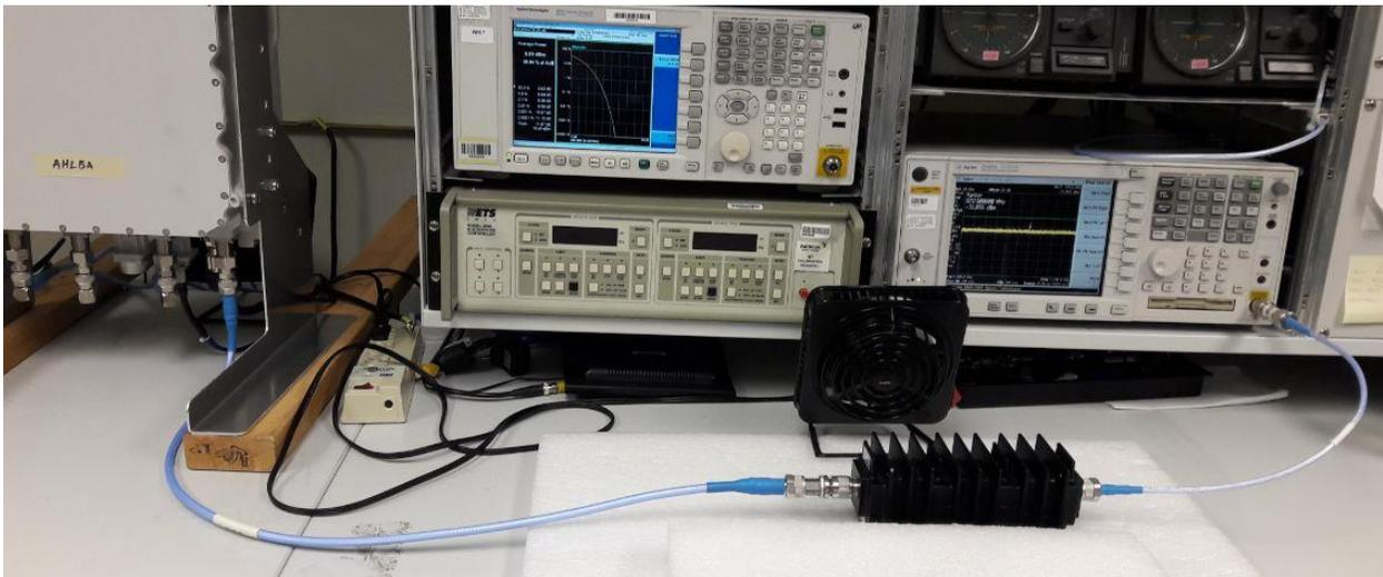
Photograph of 9kHz to 150kHz, 150kHz to 20MHz, 20MHz to 700MHz, 700MHz to 800MHz, and 800MHz to 1.1GHz Test Setup
