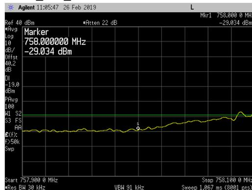
IoT Guard Band Carrier at Upper Placement
