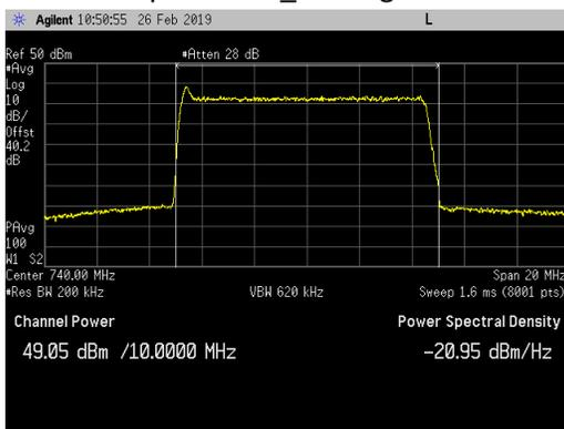
**LTE10 Channel Power Plots for a Single Narrow Band IoT Upper Guard Band Carrier:**
