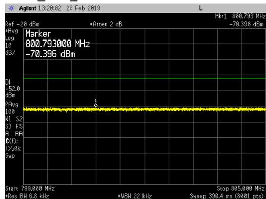
**Transmitter Antenna Port Conducted Emissions**
