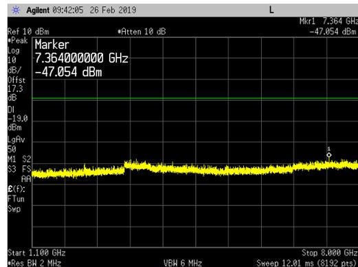
**Band 12 LTE10 Single Narrow Band IoT Upper Guard Band Carrier**
