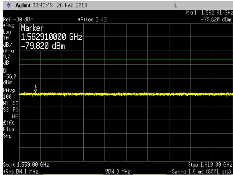
**Band 12 LTE10 Single Narrow Band IoT Upper Guard Band Carrier (Band 14 Carrier Off)**
