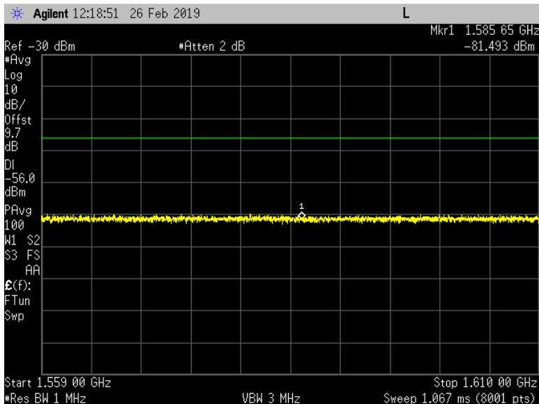
**Band 12 and Band 14 LTE10 Single Narrow Band IoT Lower Guard Band Carriers (80W/Port)**
