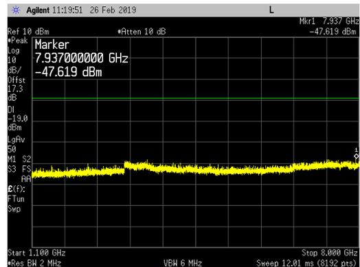
**Band 14 LTE10 Single Narrow Band IoT Upper Guard Band Carrier**
