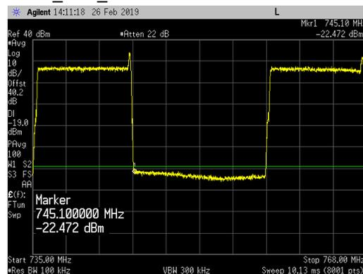
**Transmitter Antenna Port Conducted Emissions**
