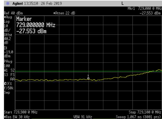
**Band 12 Single Narrow Band IoT Guard Band Carrier -Upper Band Edge Plots:**
