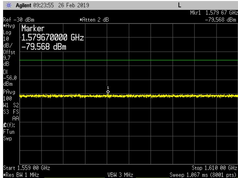
**Band 14 LTE10 Single Narrow Band IoT Lower Guard Band Carrier (Band 12 Carrier Off)**
