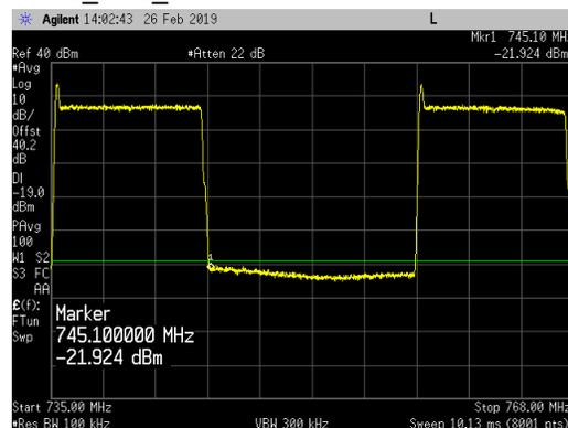
**IoT Guard Band Carrier at Upper Placement**
