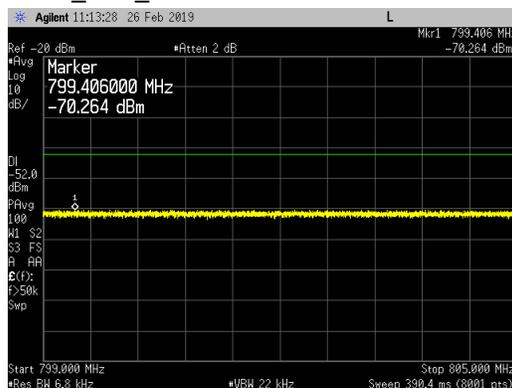
**Band 14 LTE10 at Mid Ch (763MHz) 80W Single Narrow Band IoT Guard Band Carrier -Upper Band Edge Plots:**
