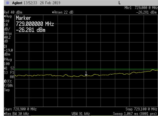
**IoT Guard Band Carrier at Upper Placement**
