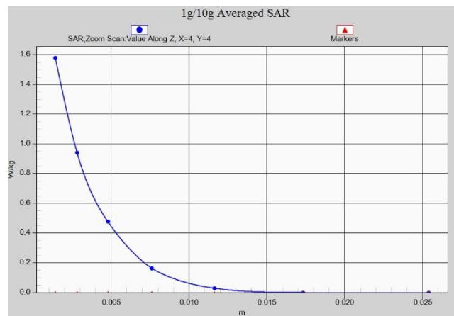
Fig. 1-27 Z-Scan at power reference point (wifi5G)
