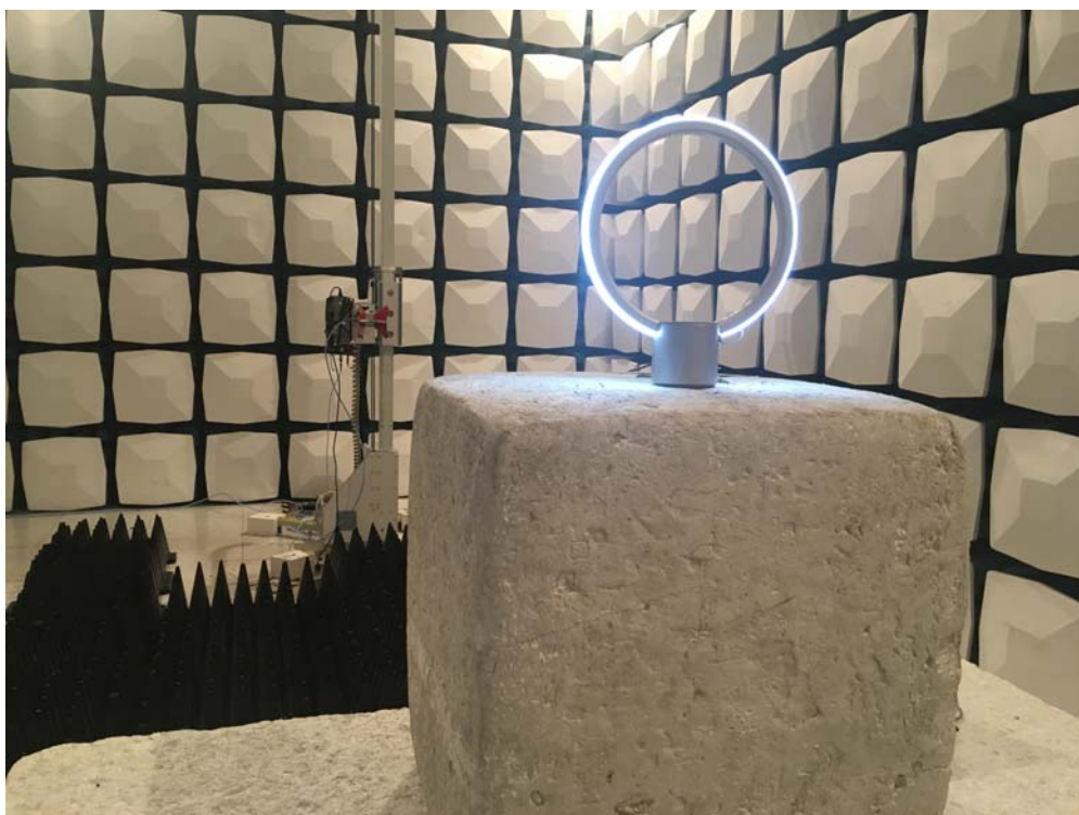
Description: Radiated Emission Test Setup for 1~18GHz
