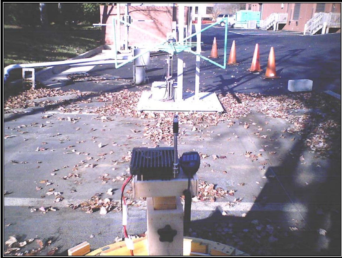
Photograph 5: Radiated Emissions Test Configuration Back View
