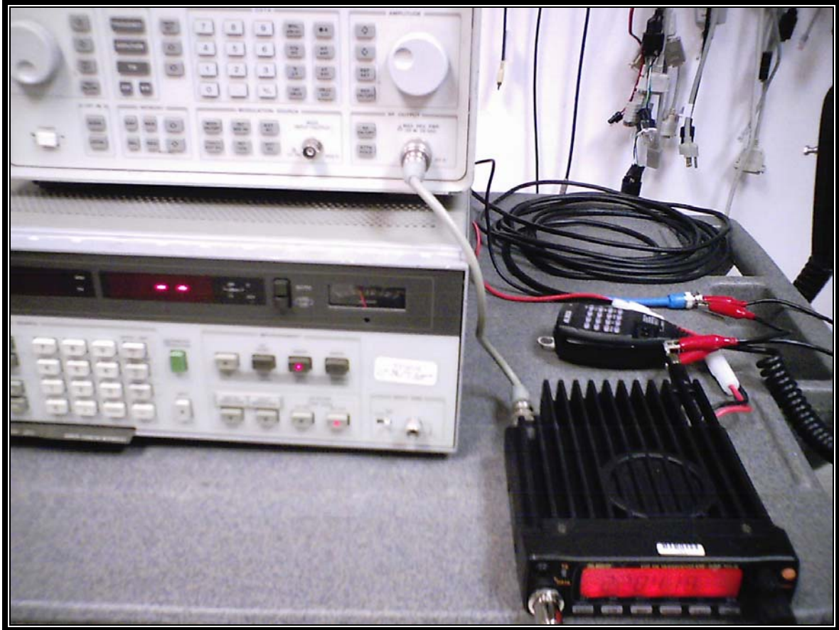
Photograph 6: 38 dB Rejection Test Setup
