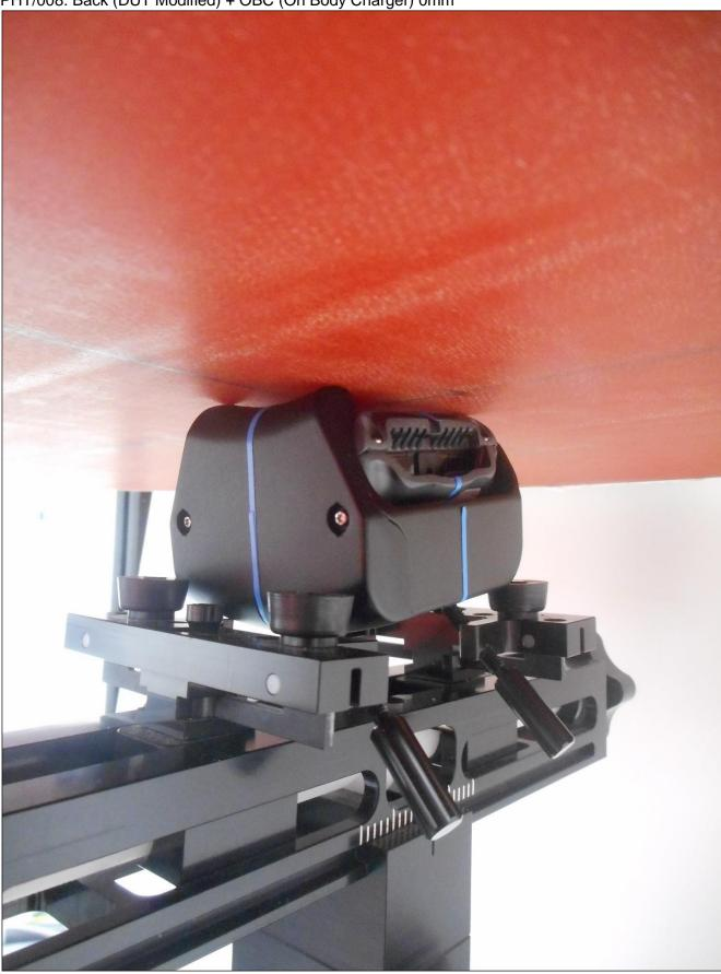
PHT/009: Edge 1 (Right) (DUT Modified) + OBC (On Body Charger) 0mm
