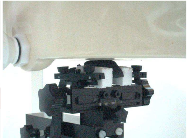
Test Position 2: Rear Face of display with 0cm Gap (2.4G WLAN)
