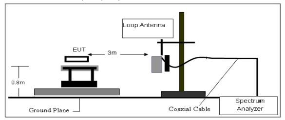
(B) Radiated Emission Test-Up Frequency 30MHz~1GHz
