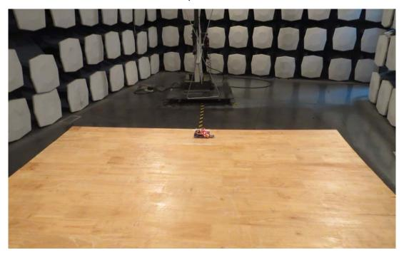
2. Above 1 GHz Radiated Emission Test Setup
