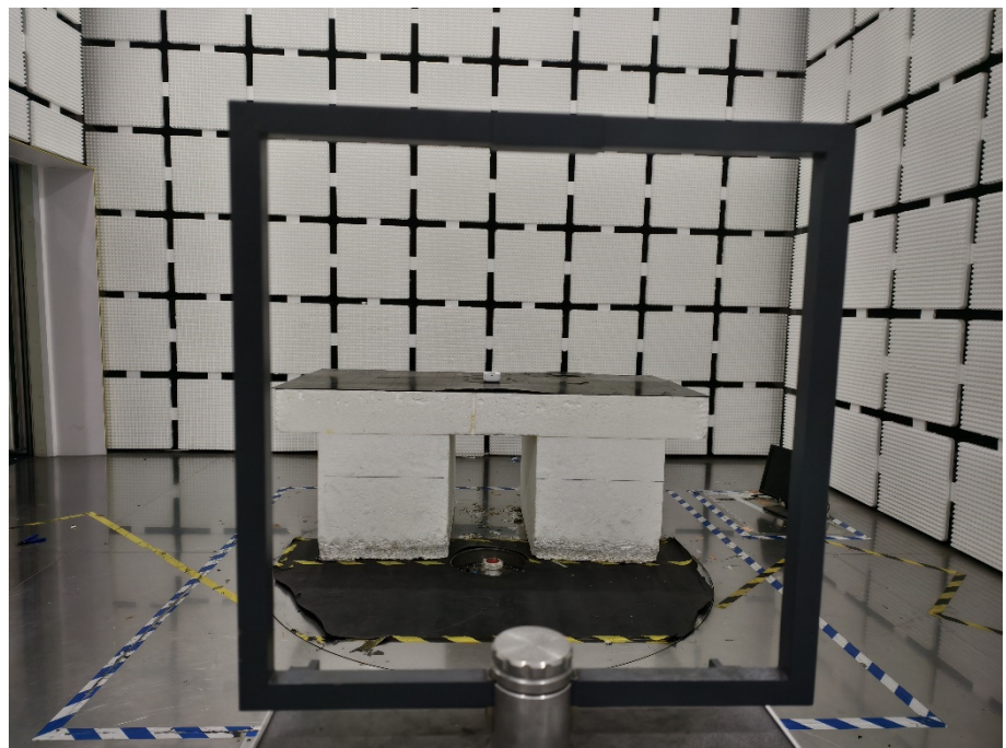
Radiation Emission Test Setup (Below 30MHz)
