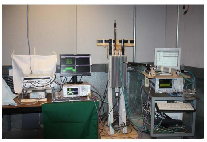
**TEST:** Measurement of Radiated Spurious Emissions
