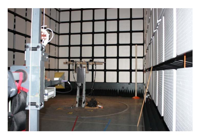
**TEST:** Measurement of Radiated Spurious Emissions
