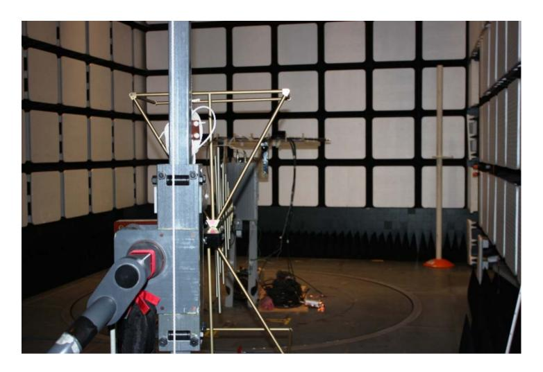
**TEST:** Measurement of Radiated Spurious Emissions
