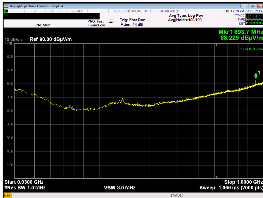
Plot 3.6.10: Spurious Emissions test results, 30 MHz – 1GHz range, Vertical polarization, High Frequency
