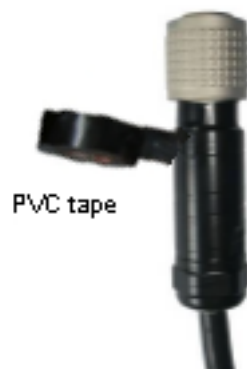
Figure 5-120 Wrapping three layers of the PVC tape
