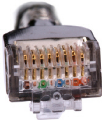
Figure 5-79 Contact strips of different heights
