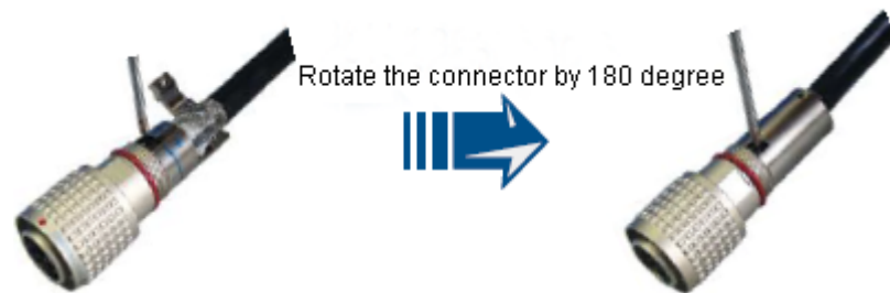
Figure 5-5 Tightening the crimping screws
