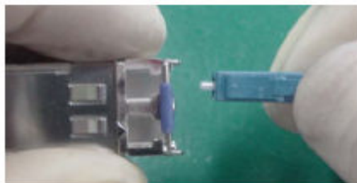
Figure 5-171 Using fibers to protect an optical module
