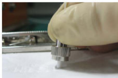
Figure 5-169 Cleaning optical fibers with special cleaning tissues
