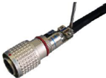
Figure 5-6 Compacting the shield layer
