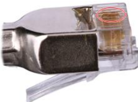
Figure 5-81 Unparallel contact strips of different heights
