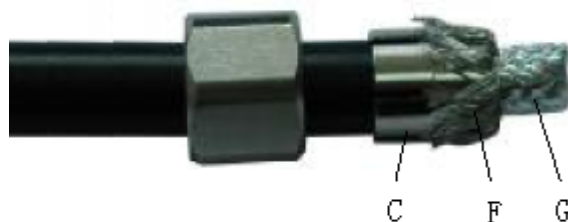
Figure 5-100 Peeling off the shielded layer
