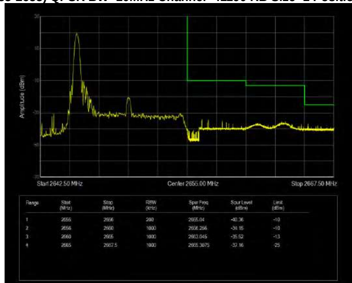
Band41(2535-2655) QPSK BW=10MHz Channel=41190 RB Size=1 Position=#Max Extended
