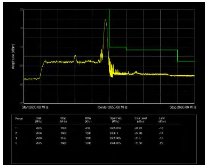
Band41(2535-2655) QPSK BW=20MHz Channel=41140 RB Size=100 Position=#0 Extended
