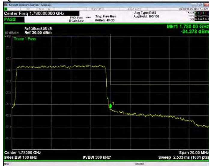
Band66 QPSK BW=15MHz Channel=132047 RB Size=1 Position=#0 Extended
