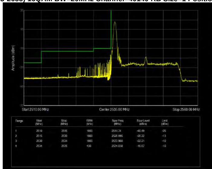
Band41(2535-2655) 16QAM BW=20MHz Channel=40140 RB Size=1 Position=#Max Extended
