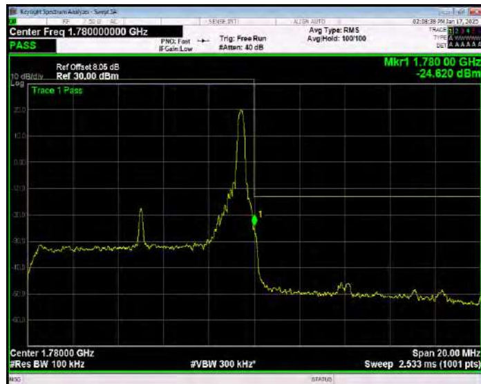
Band66 16QAM BW=10MHz Channel=132622 RB Size=50 Position=#0 Extended
