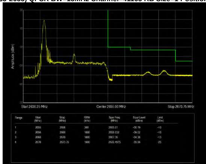
Band41(2535-2655) QPSK BW=15MHz Channel=41165 RB Size=1 Position=#Max Extended
