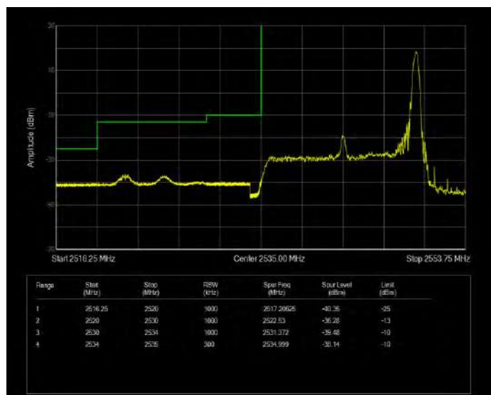
Band41(2535-2655) 16QAM BW=15MHz Channel=40115 RB Size=75 Position=#0 Extended
