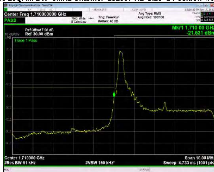
Band66 16QAM BW=5MHz Channel=131997 RB Size=1 Position=#Max Extended
