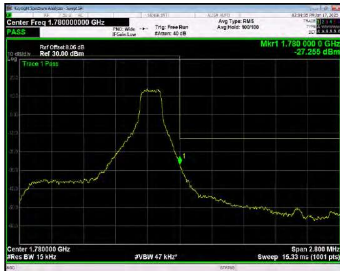
Band66 QPSK BW=1.4MHz Channel=132665 RB Size=6 Position=#0 Extended
