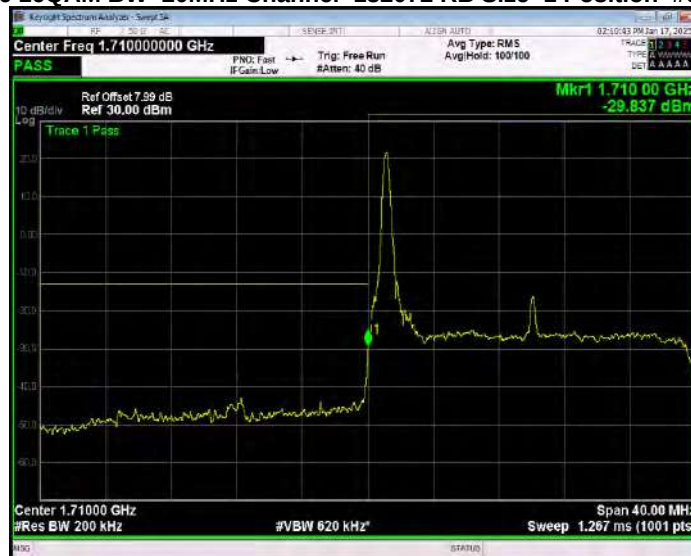
Band66 16QAM BW=20MHz Channel=132072 RB Size=1 Position=#Max Extended
