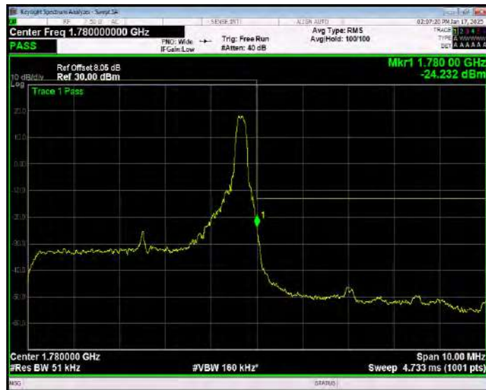
Band66 16QAM BW=5MHz Channel=132647 RB Size=25 Position=#0 Extended
