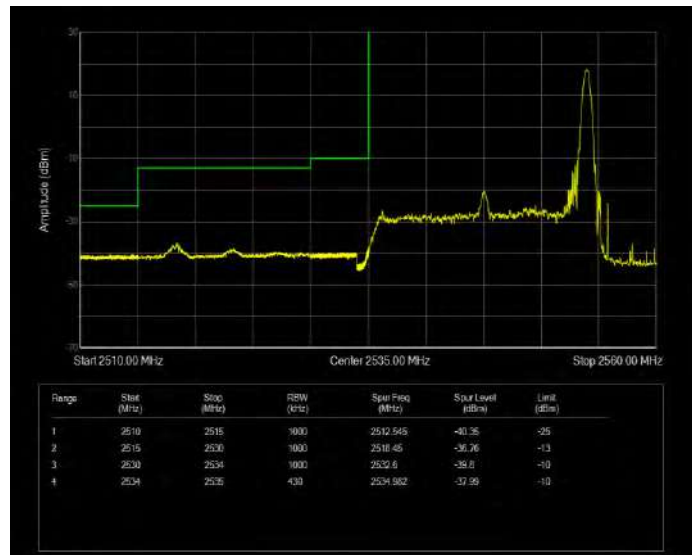
Band41(2535-2655) 16QAM BW=20MHz Channel=40140 RB Size=100 Position=#0 Extended
