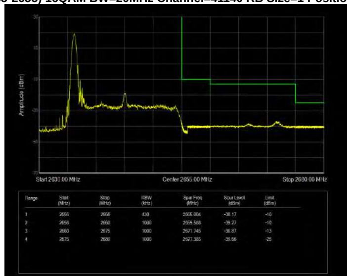
Band41(2535-2655) 16QAM BW=20MHz Channel=41140 RB Size=1 Position=#Max Extended
