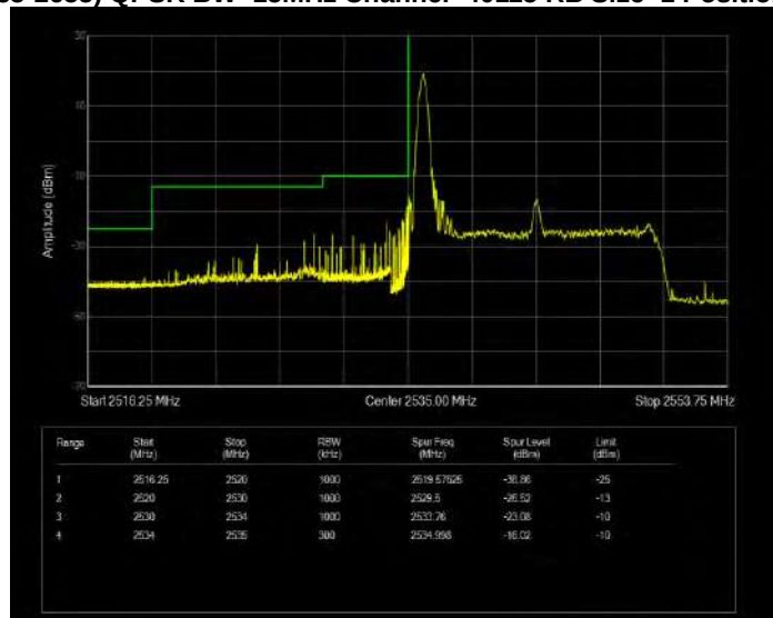
Band41(2535-2655) QPSK BW=15MHz Channel=40115 RB Size=1 Position=#Max Extended
