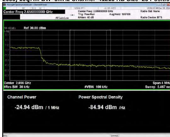
Band41(2535-2655) 16QAM BW=5MHz Channel=41215 RB Size=25 Position=#0 Normal
