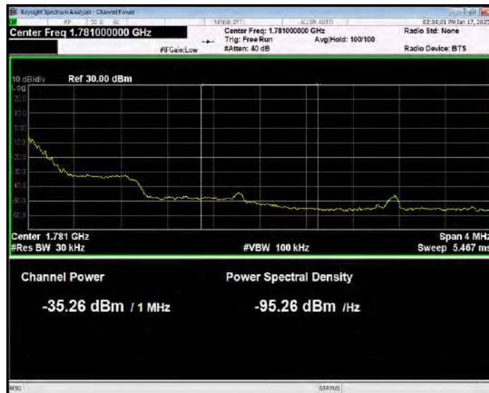
Band66 QPSK BW=1.4MHz Channel=132665 RB Size=1 Position=#0 Normal
