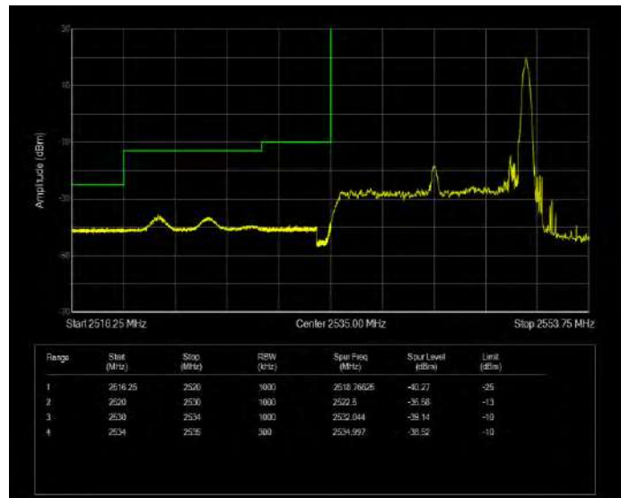
Band41(2535-2655) QPSK BW=15MHz Channel=40115 RB Size=75 Position=#0 Extended
