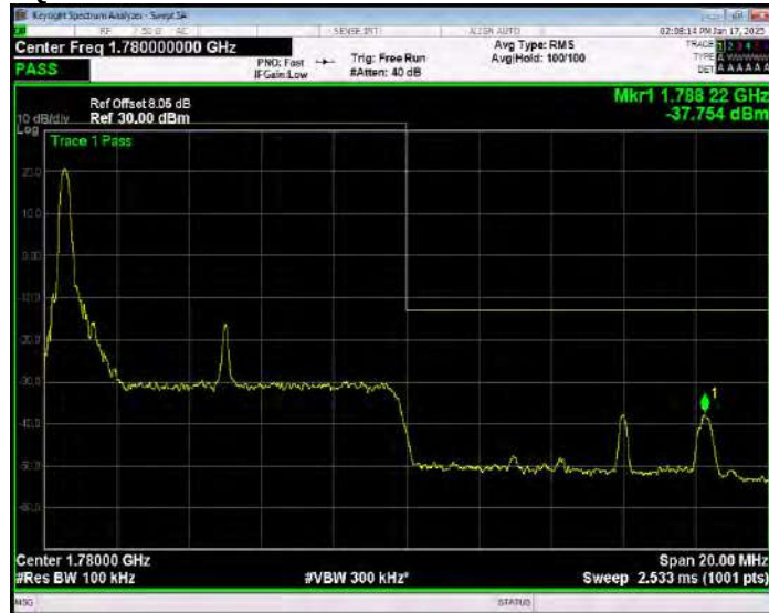
Band66 QPSK BW=10MHz Channel=132622 RB Size=1 Position=#Max Extended
