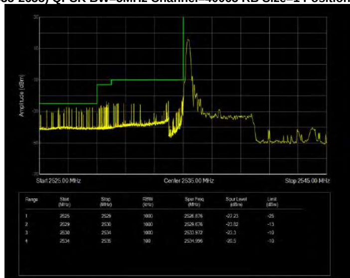
Band41(2535-2655) QPSK BW=5MHz Channel=40065 RB Size=1 Position=#Max Extended
