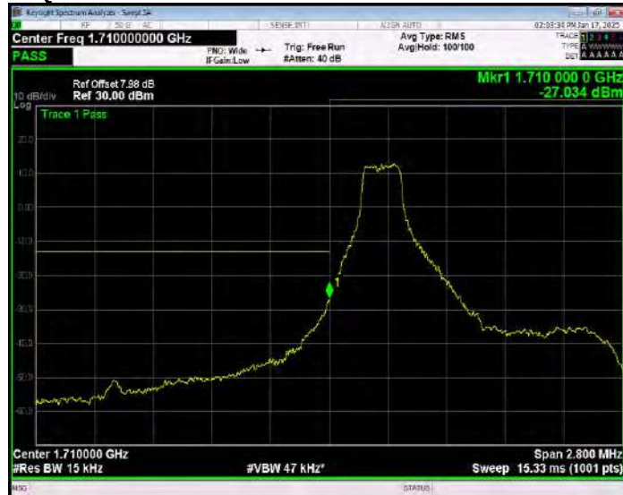
Band66 16QAM BW=1.4MHz Channel=131979 RB Size=1 Position=#Max Extended
