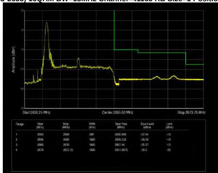
Band41(2535-2655) 16QAM BW=15MHz Channel=41165 RB Size=1 Position=#Max Extended
