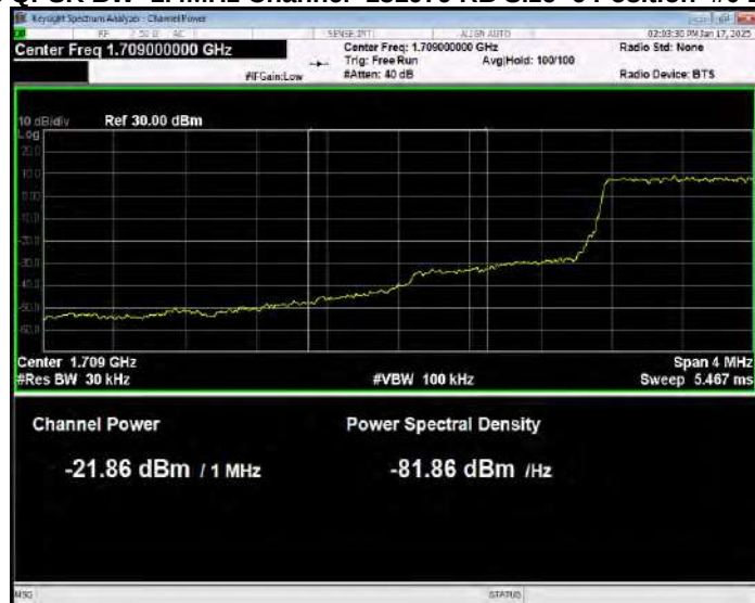
Band66 QPSK BW=1.4MHz Channel=131979 RB Size=6 Position=#0 Normal
