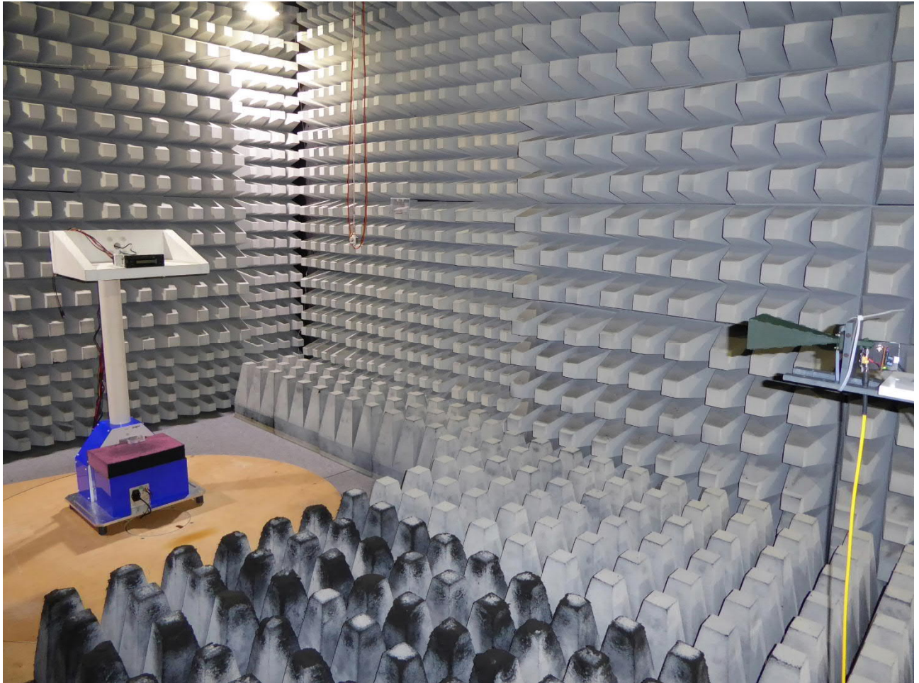
Test setup fully anechoic chamber (12 - 18 GHz)
