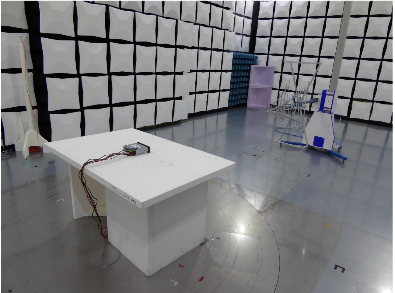
Test setup semi anechoic chamber (30 MHz – 1 GHz)
