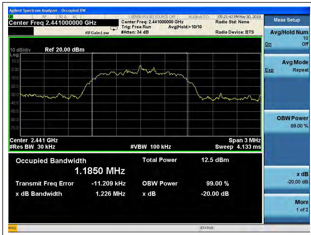
( \pi/4 -DQPSK, Channel 39, 2441MHz)
