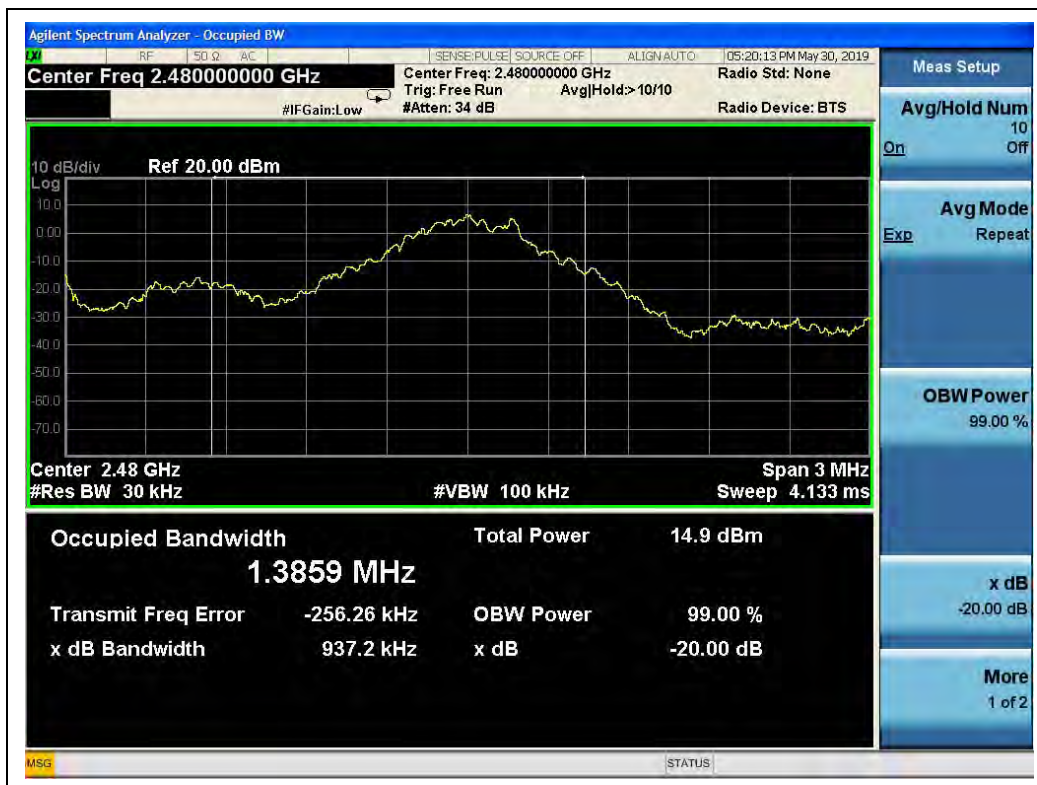
(GFSK, Channel 78, 2480MHz)
