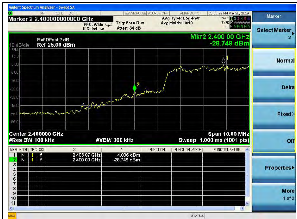
(Channel = 0, Band edge with hopping on, 8-DPSK)
