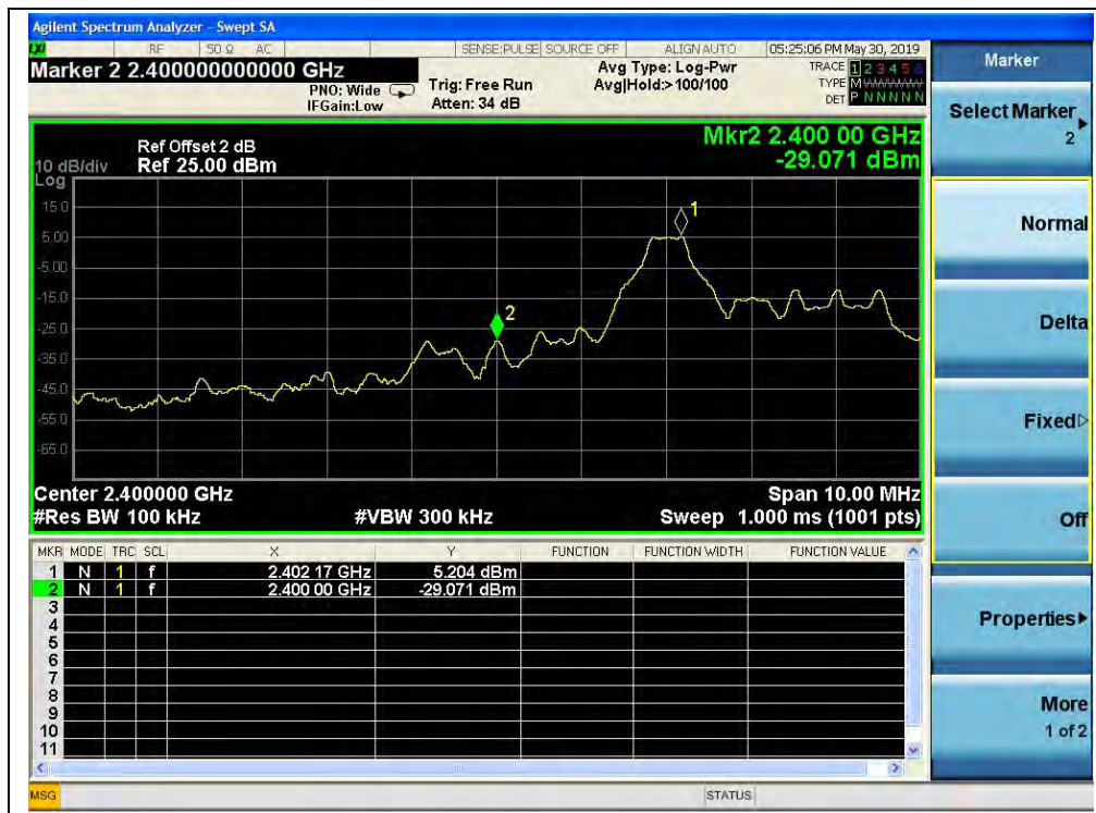
(Channel = 0, Band edge, GFSK Mode)
