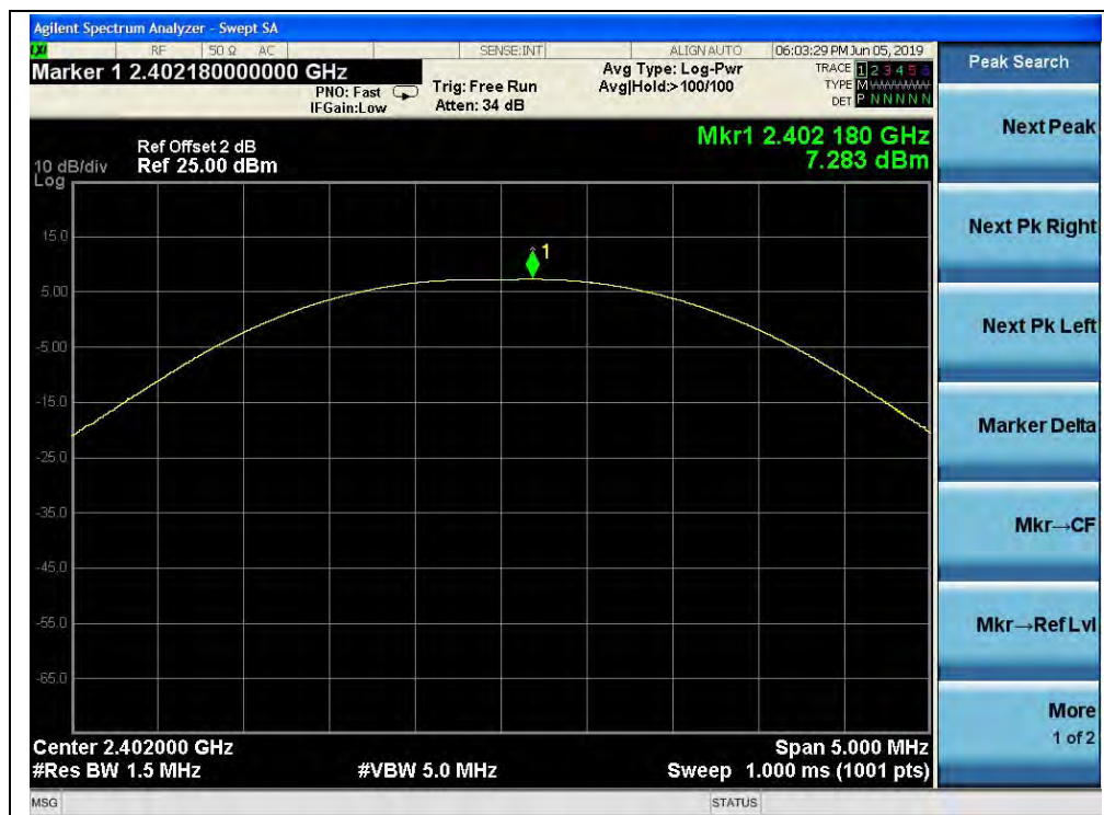
(GFSK, Channel 0, 2402MHz)
