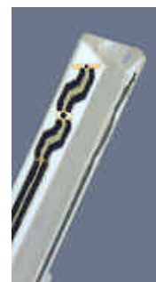
Figure 3.2 Probe Thick-Film Technique
