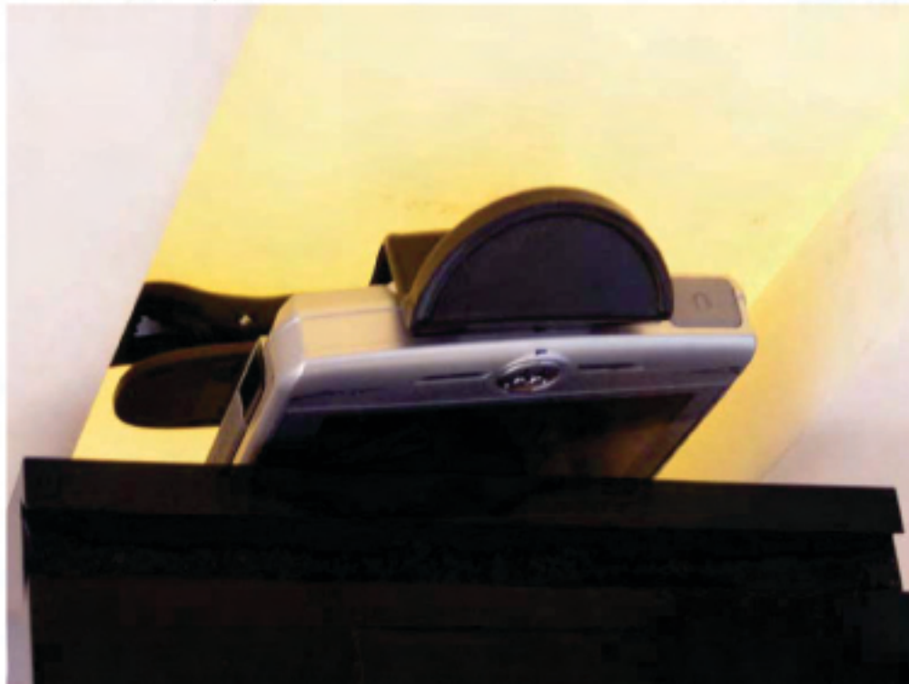
Figure 5: Phone Against the Flat Phantom with Slim Holster
