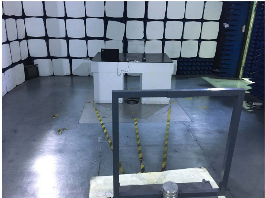
Radiation Emission Test Setup (Below 30MHz)
