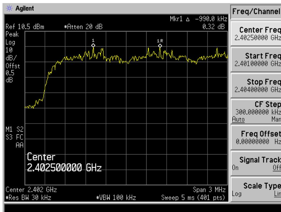
Channel Spacing (Middle CH=1MHz)
