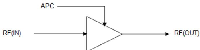
There is a transmission power table about PCLS and APC\_DAC, by adjusting the voltage value of the APC, to change the transmission power.
