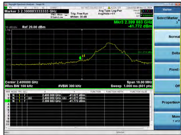
GFSK LOW CHANNEL, BAND EDGE
