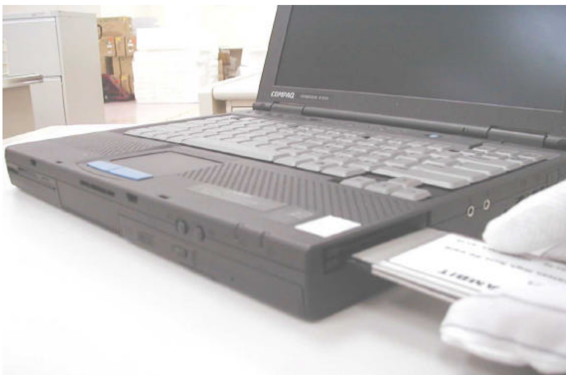
Figure2. Insert the Wireless High Rate PC Card into a PCMCIA slot.
