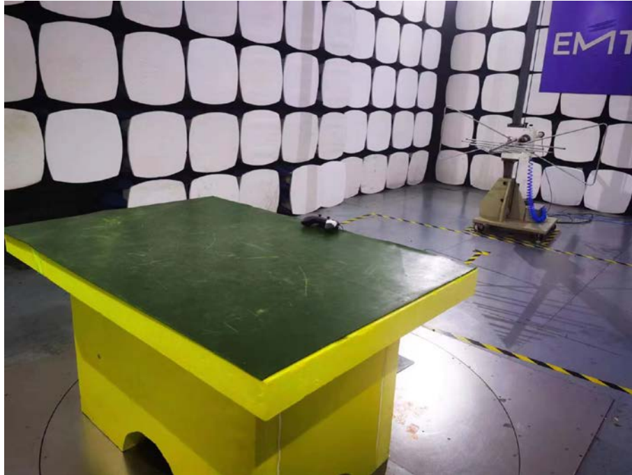
Spurious Emission Test Setup (Above 1GHz)
