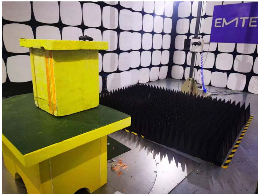
Spurious Emission Test Setup (Above 1GHz)
