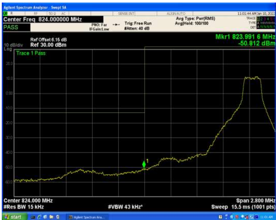
Band5 QAM16 BW=1.4MHz Channel=20643 RB Size=1 Position=#Max
