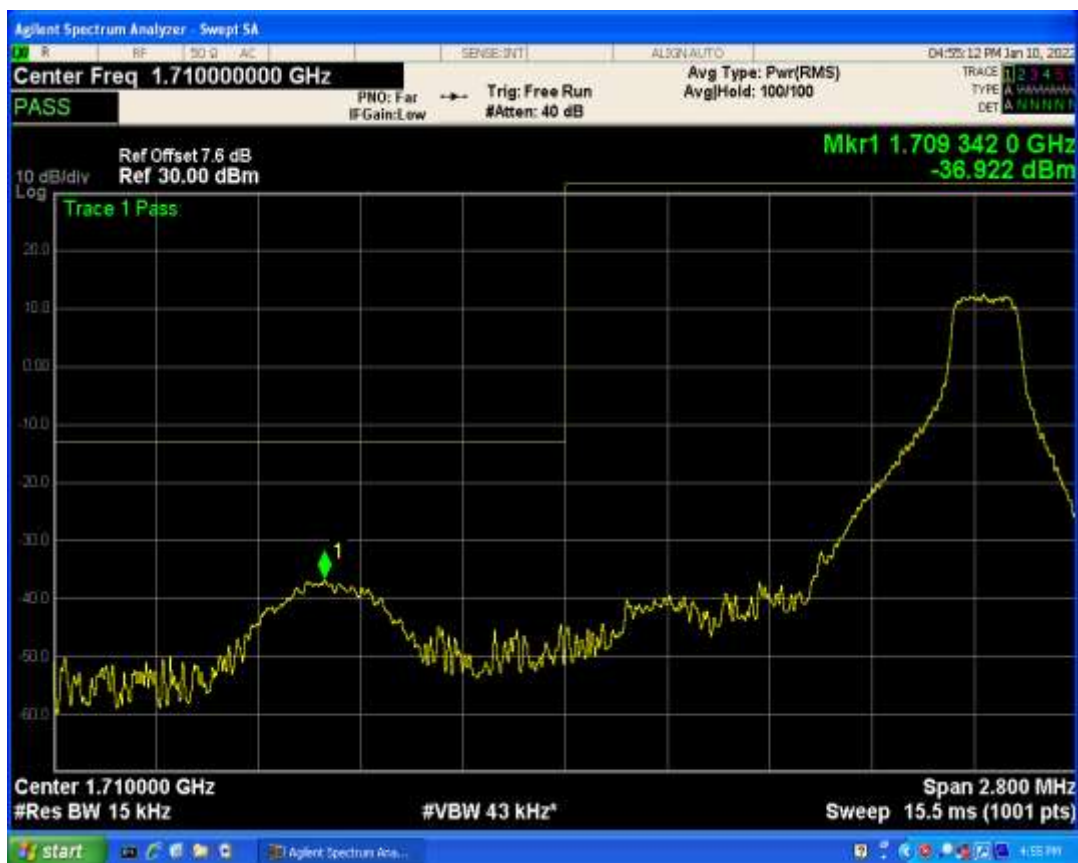
Band66 QPSK BW=1.4MHz Channel=132665 RB Size=1 Position=#0
