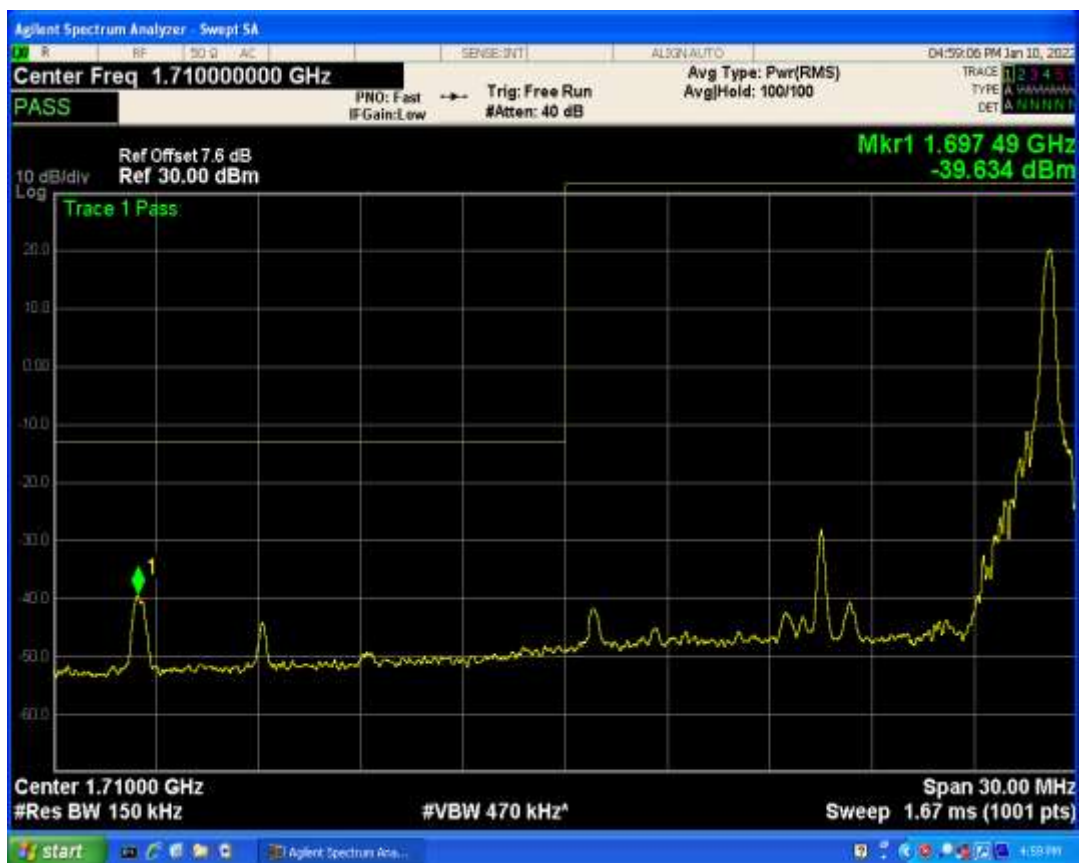
Band66 QAM16 BW=15MHz Channel=132597 RB Size=1 Position=#0
