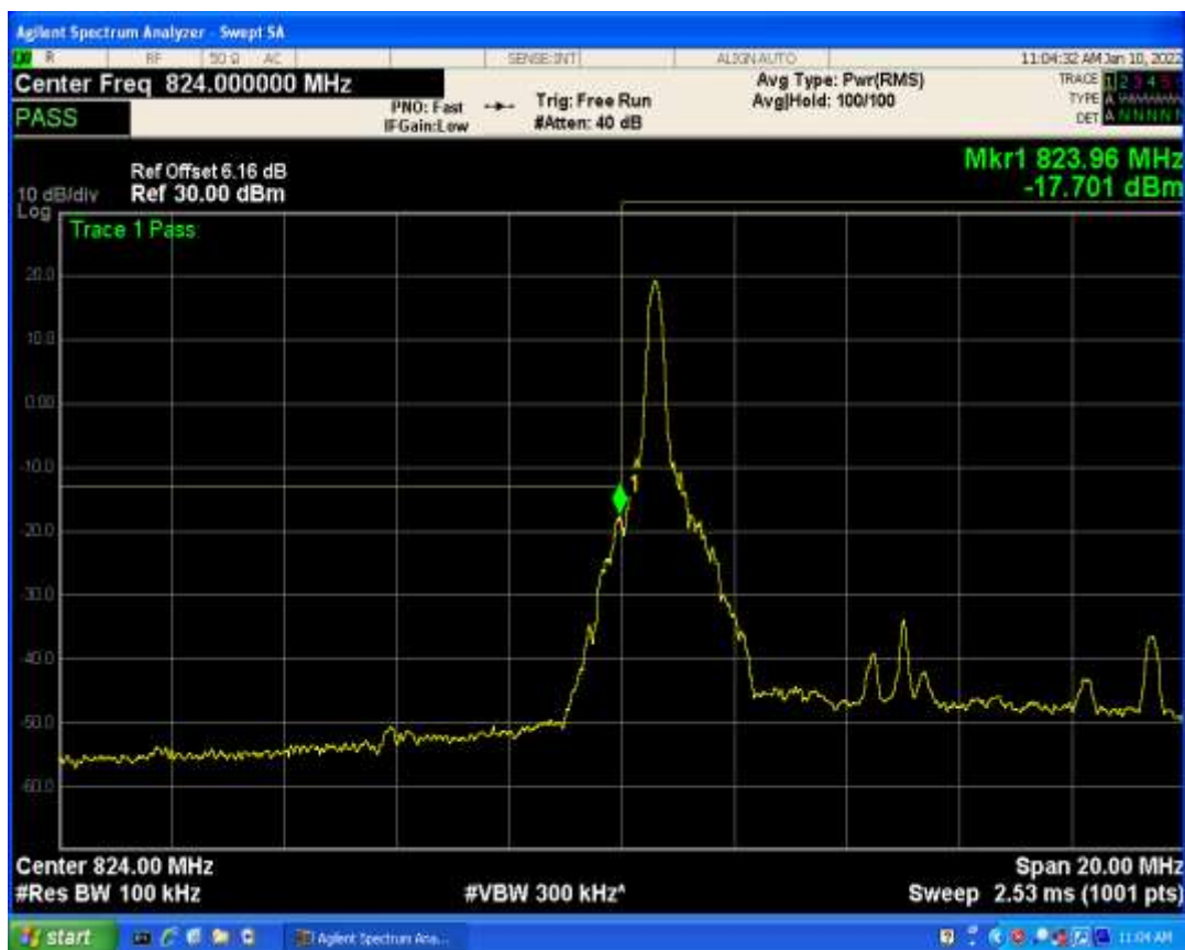
Band5 QAM16 BW=10MHz Channel=20600 RB Size=1 Position=#0
