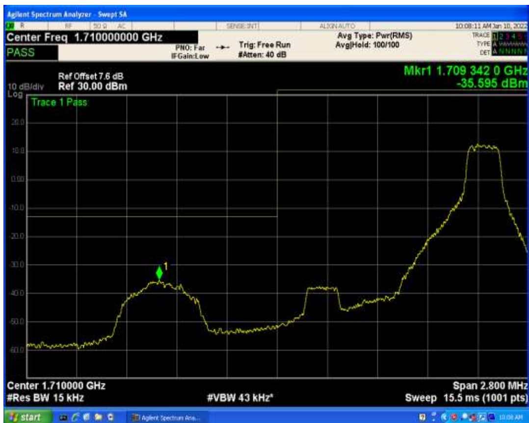
Band4 QPSK BW=15MHz Channel=20025 RB Size=75 Position=#0
