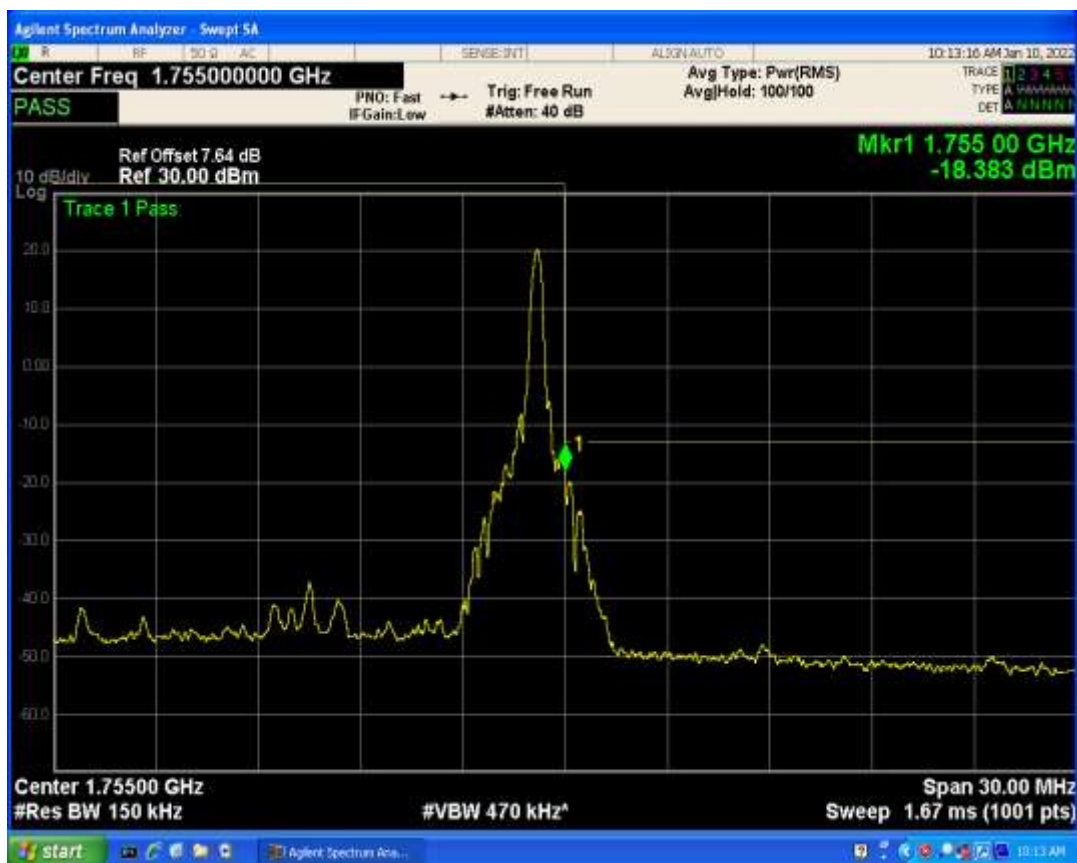
Band4 QAM16 BW=5MHz Channel=19975 RB Size=1 Position=#0
