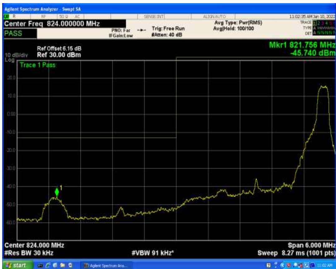
Band5 QPSK BW=3MHz Channel=20635 RB Size=1 Position=#0
