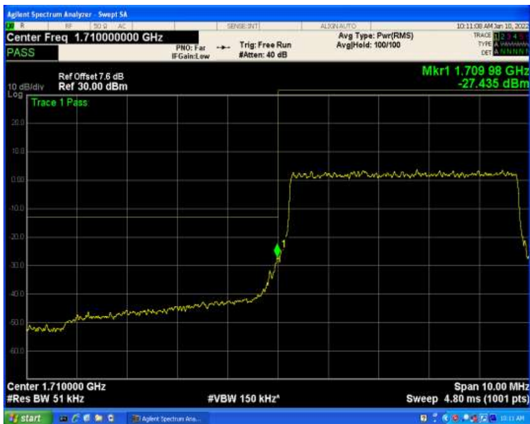
Band4 QPSK BW=5MHz Channel=20375 RB Size=25 Position=#0
