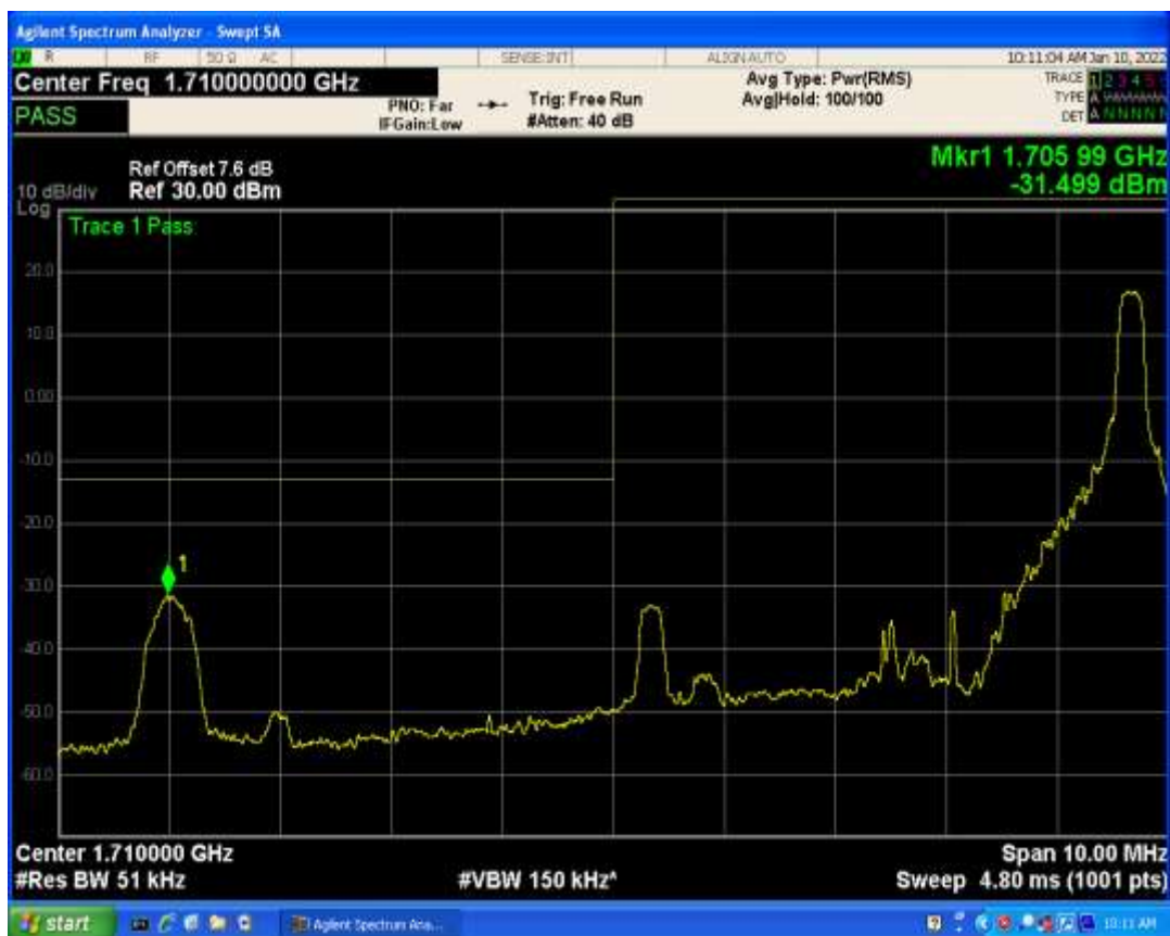
Band4 QPSK BW=3MHz Channel=20385 RB Size=1 Position=#Max
