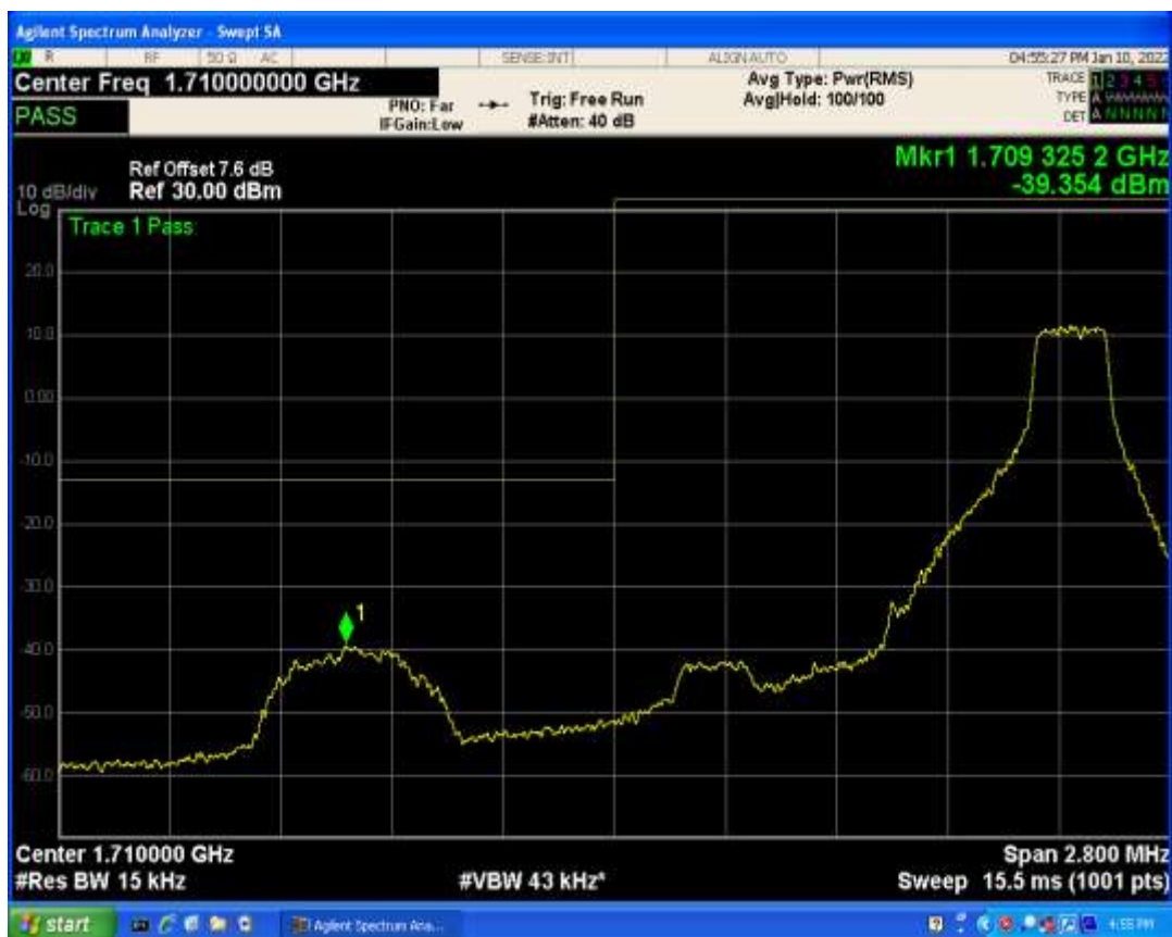
Band66 QAM16 BW=1.4MHz Channel=132665 RB Size=1 Position=#0
