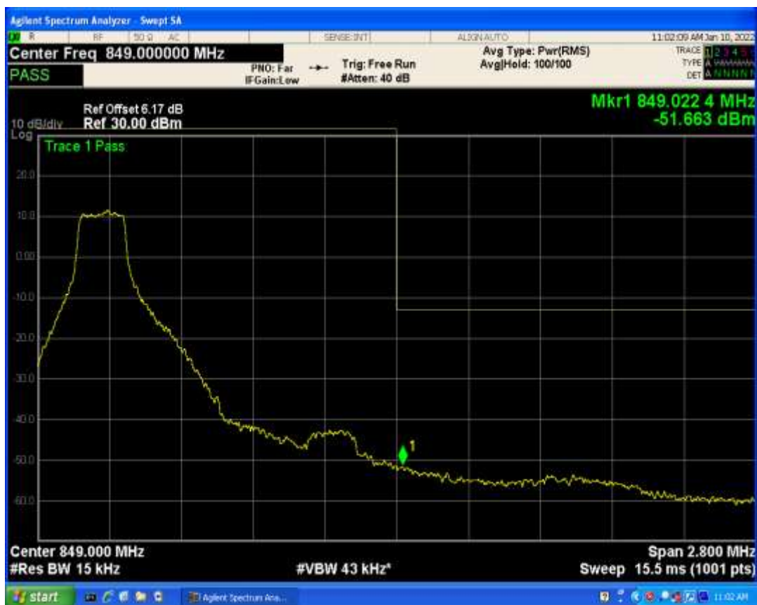
Band5 QAM16 BW=3MHz Channel=20635 RB Size=1 Position=#Max
