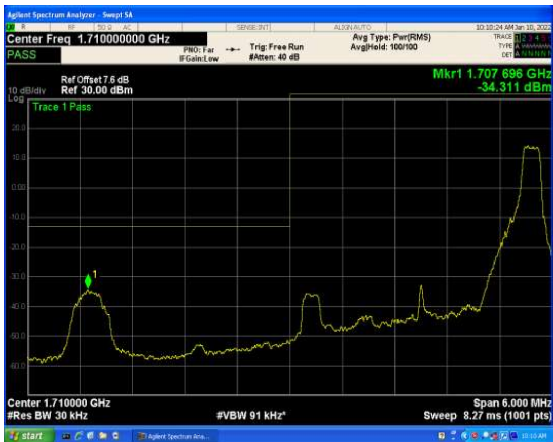
Band4 QAM16 BW=3MHz Channel=20385 RB Size=1 Position=#0
