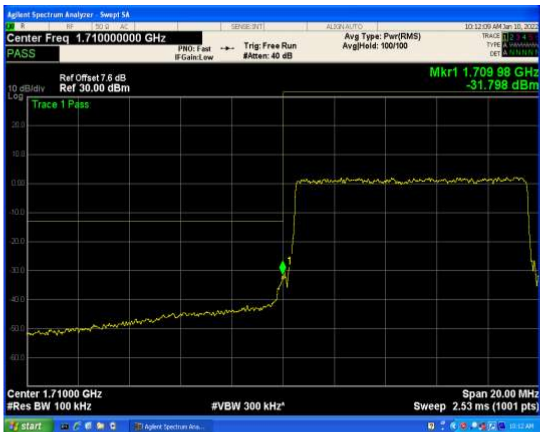
Band4 QAM16 BW=10MHz Channel=20350 RB Size=1 Position=#0
