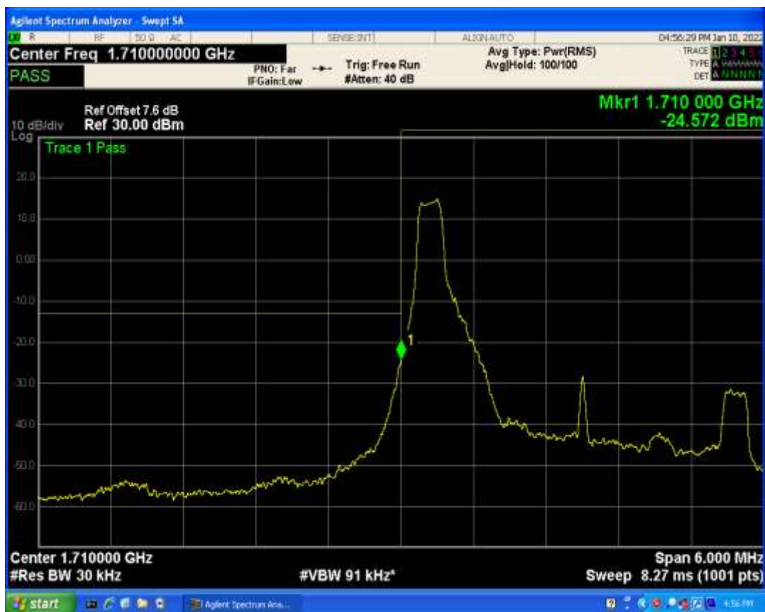
Band66 QPSK BW=1.4MHz Channel=131979 RB Size=6 Position=#0
