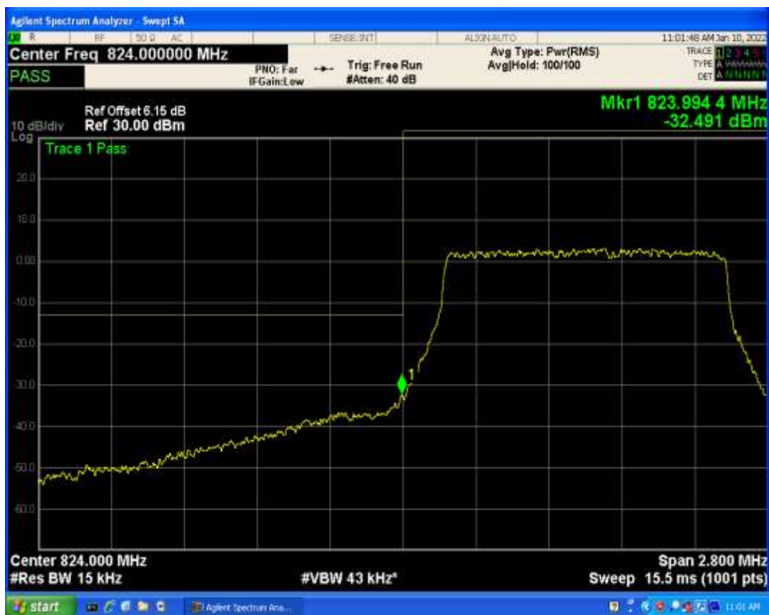
Band5 QAM16 BW=1.4MHz Channel=20407 RB Size=1 Position=#Max
