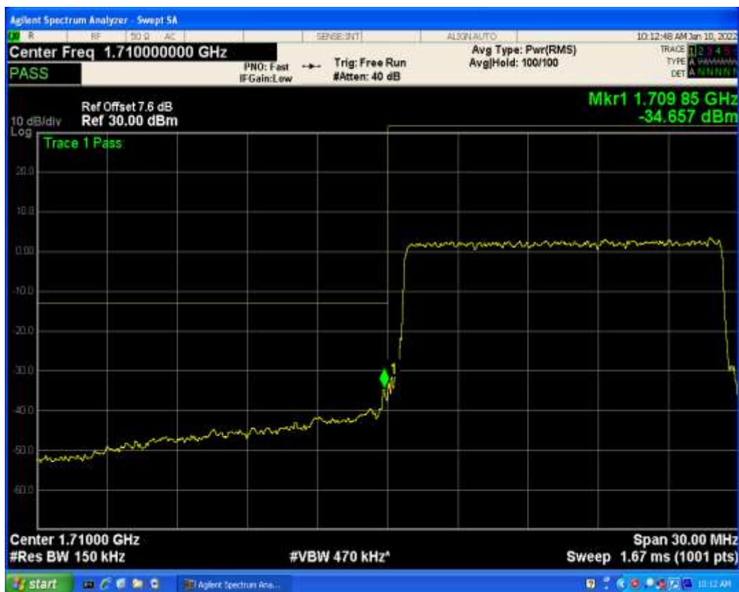
Band4 QPSK BW=15MHz Channel=20025 RB Size=1 Position=#Max
