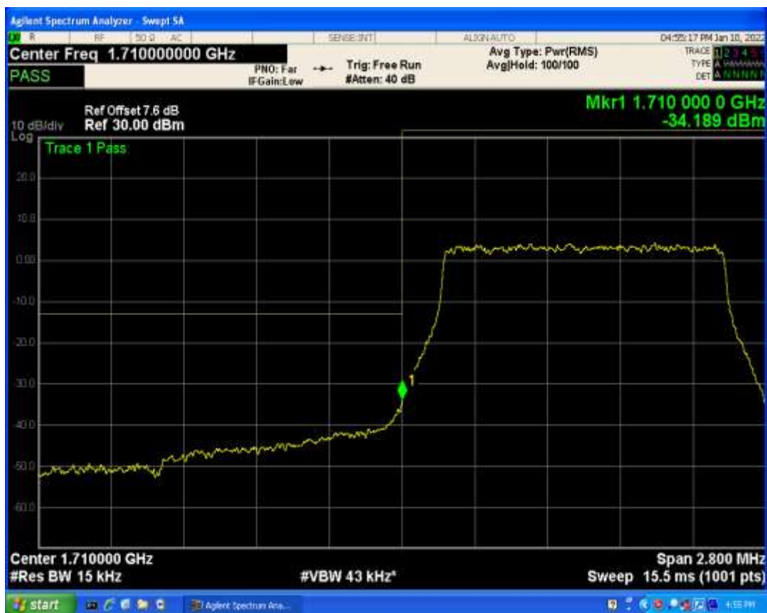
Band66 QPSK BW=1.4MHz Channel=131979 RB Size=1 Position=#Max
