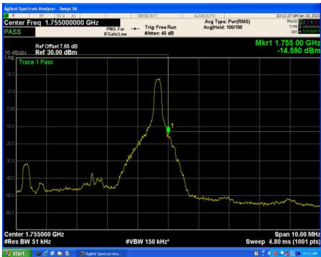
Band4 QPSK BW=5MHz Channel=19975 RB Size=1 Position=#Max
