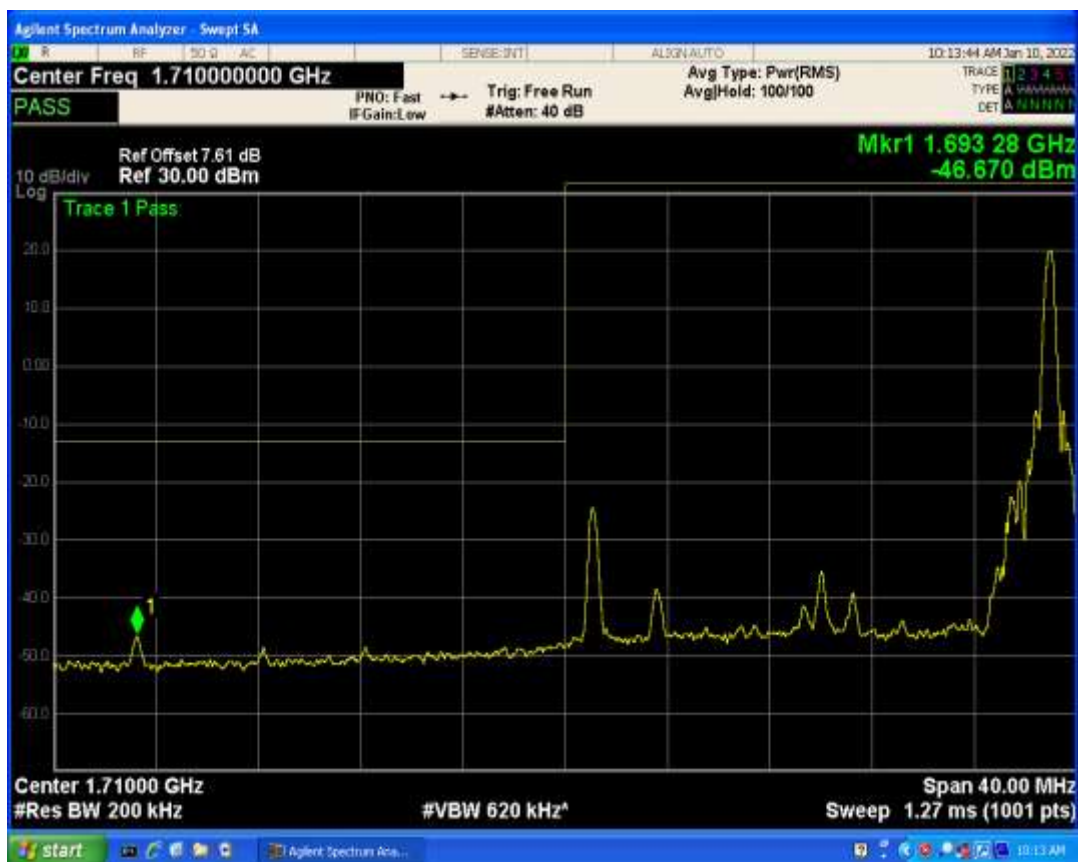
Band4 QAM16 BW=20MHz Channel=20050 RB Size=1 Position=#0
