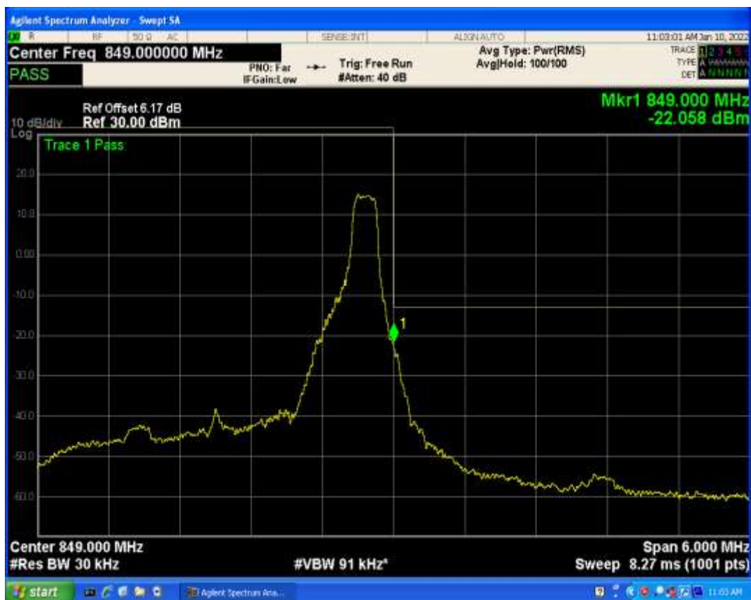
Band5 QPSK BW=5MHz Channel=20425 RB Size=1 Position=#Max
