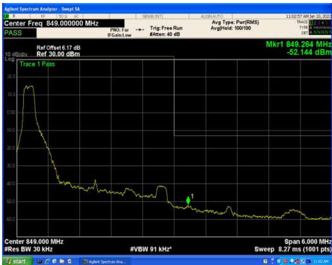
Band5 QPSK BW=3MHz Channel=20415 RB Size=15 Position=#0
