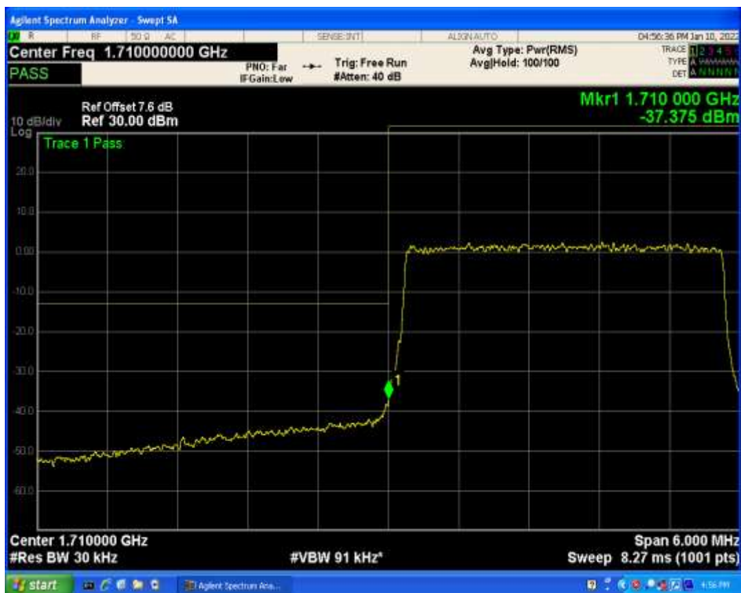
Band66 QAM16 BW=3MHz Channel=132657 RB Size=1 Position=#Max
