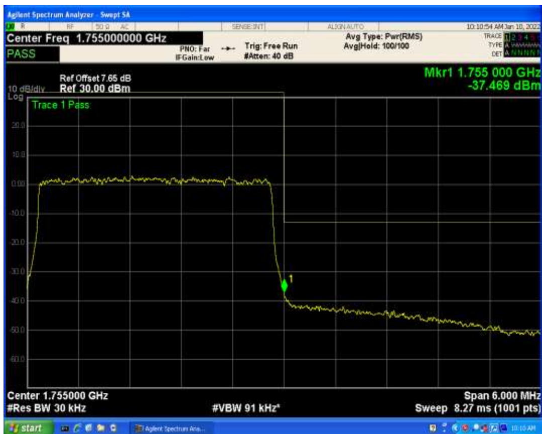
Band4 QAM16 BW=5MHz Channel=19975 RB Size=1 Position=#Max
