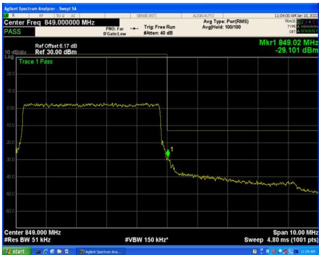
Band5 QPSK BW=5MHz Channel=20625 RB Size=1 Position=#Max
