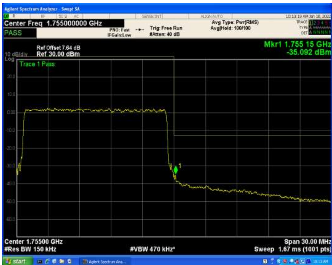
Band4 QAM16 BW=15MHz Channel=20325 RB Size=1 Position=#Max
