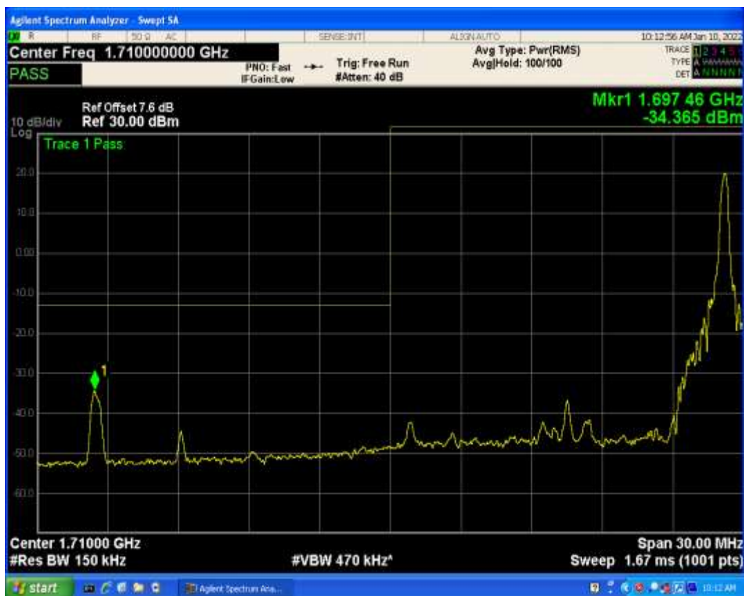
Band4 QAM16 BW=15MHz Channel=20325 RB Size=1 Position=#0
