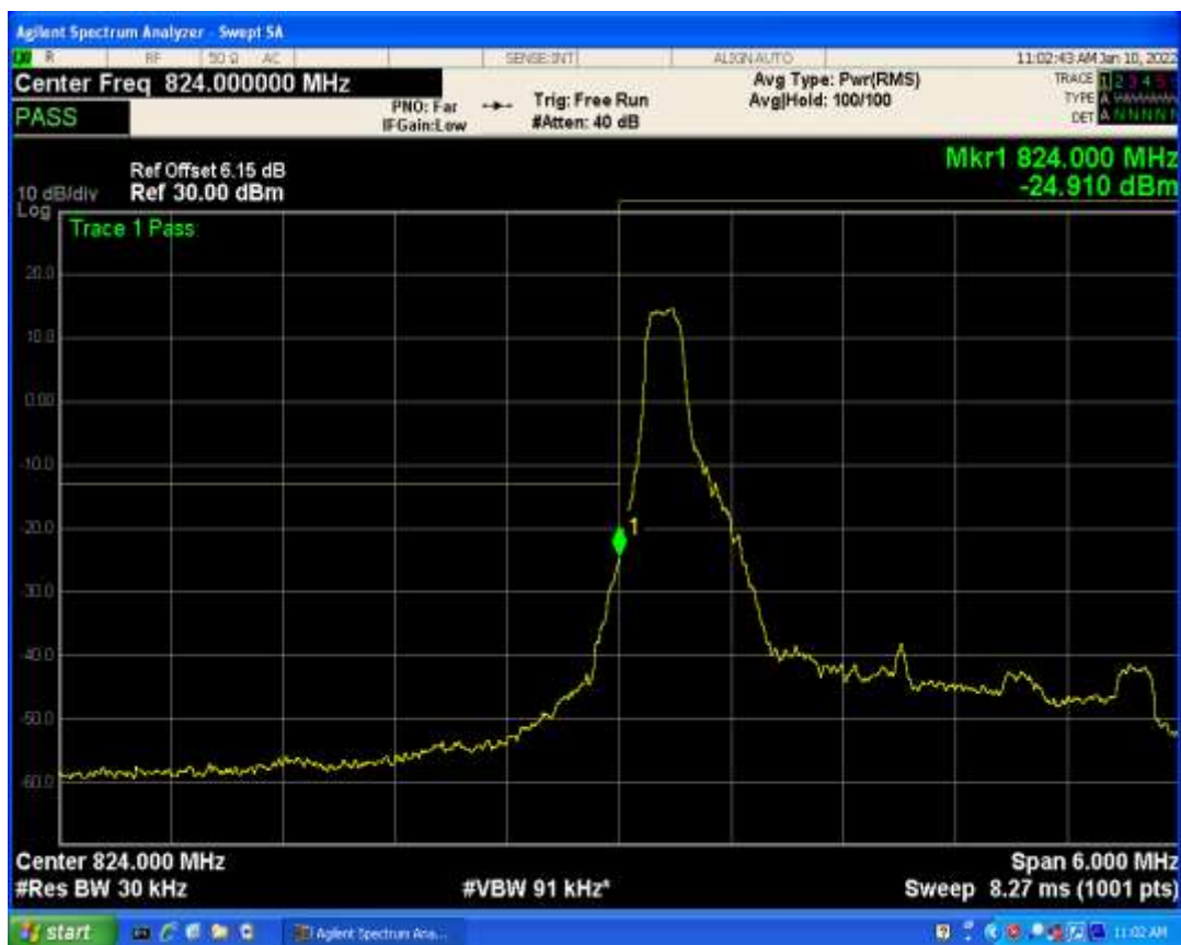
Band5 QPSK BW=1.4MHz Channel=20407 RB Size=6 Position=#0
