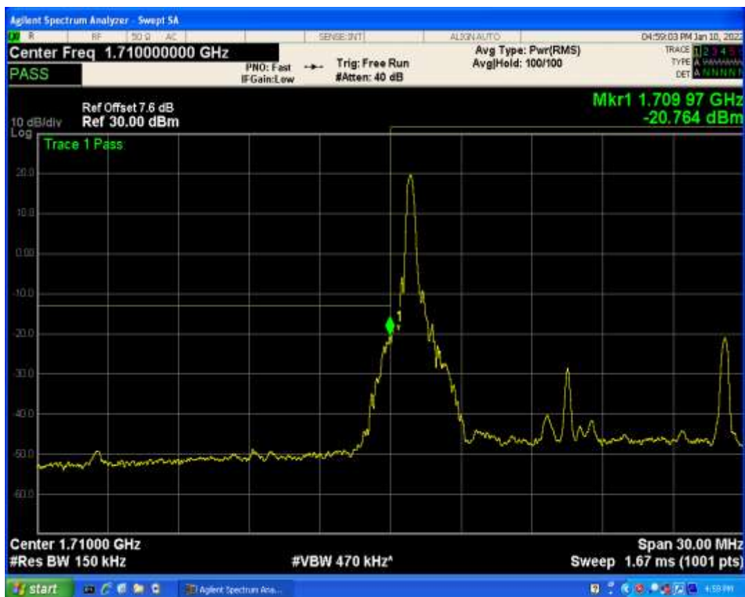
Band66 QAM16 BW=10MHz Channel=132622 RB Size=50 Position=#0
