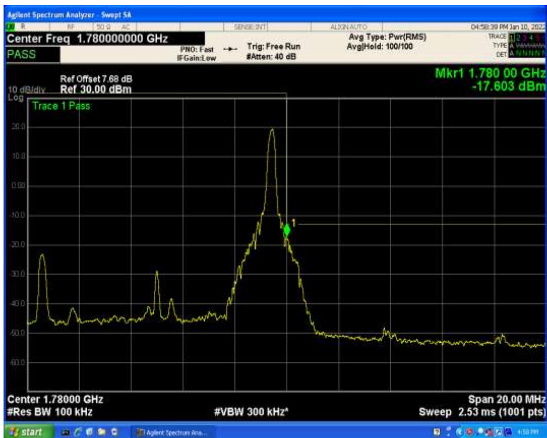
Band66 QAM16 BW=10MHz Channel=132622 RB Size=1 Position=#0
