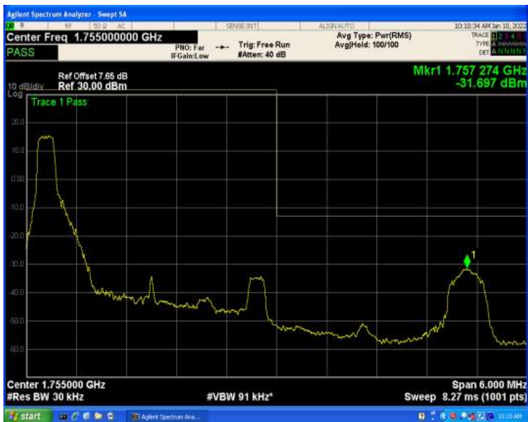
Band4 QPSK BW=5MHz Channel=19975 RB Size=1 Position=#0
