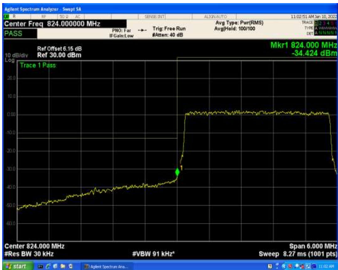
Band5 QAM16 BW=10MHz Channel=20600 RB Size=50 Position=#0
