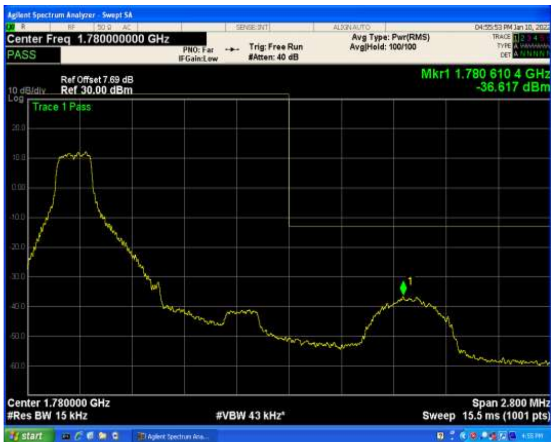
Band66 QAM16 BW=1.4MHz Channel=132665 RB Size=6 Position=#0
