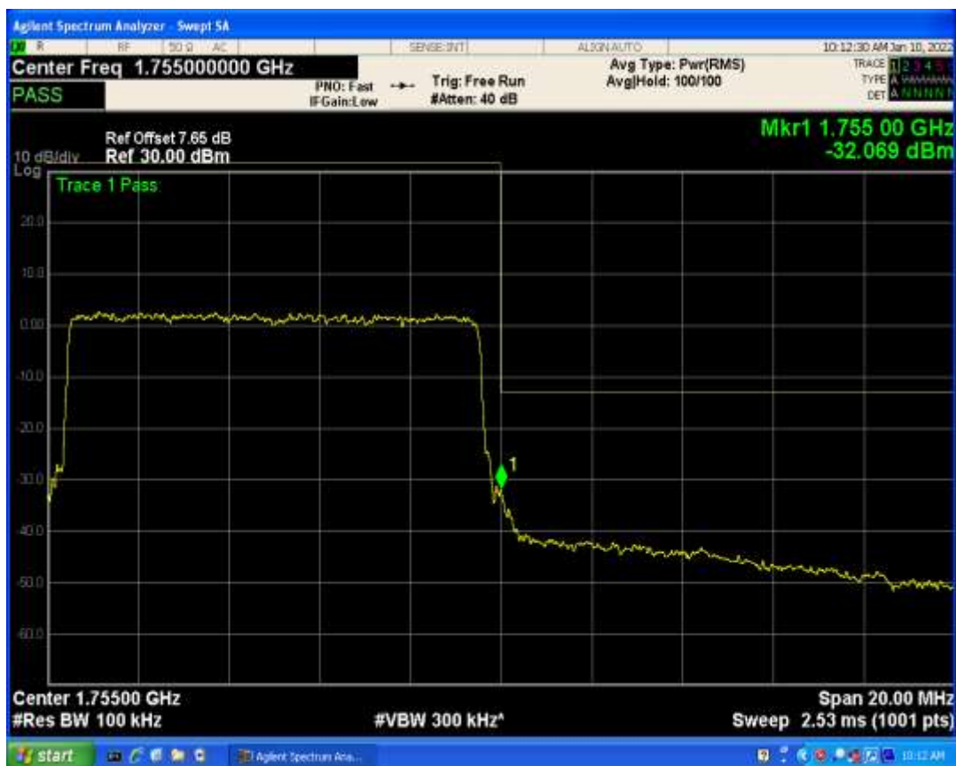
Band4 QAM16 BW=15MHz Channel=20025 RB Size=1 Position=#0
