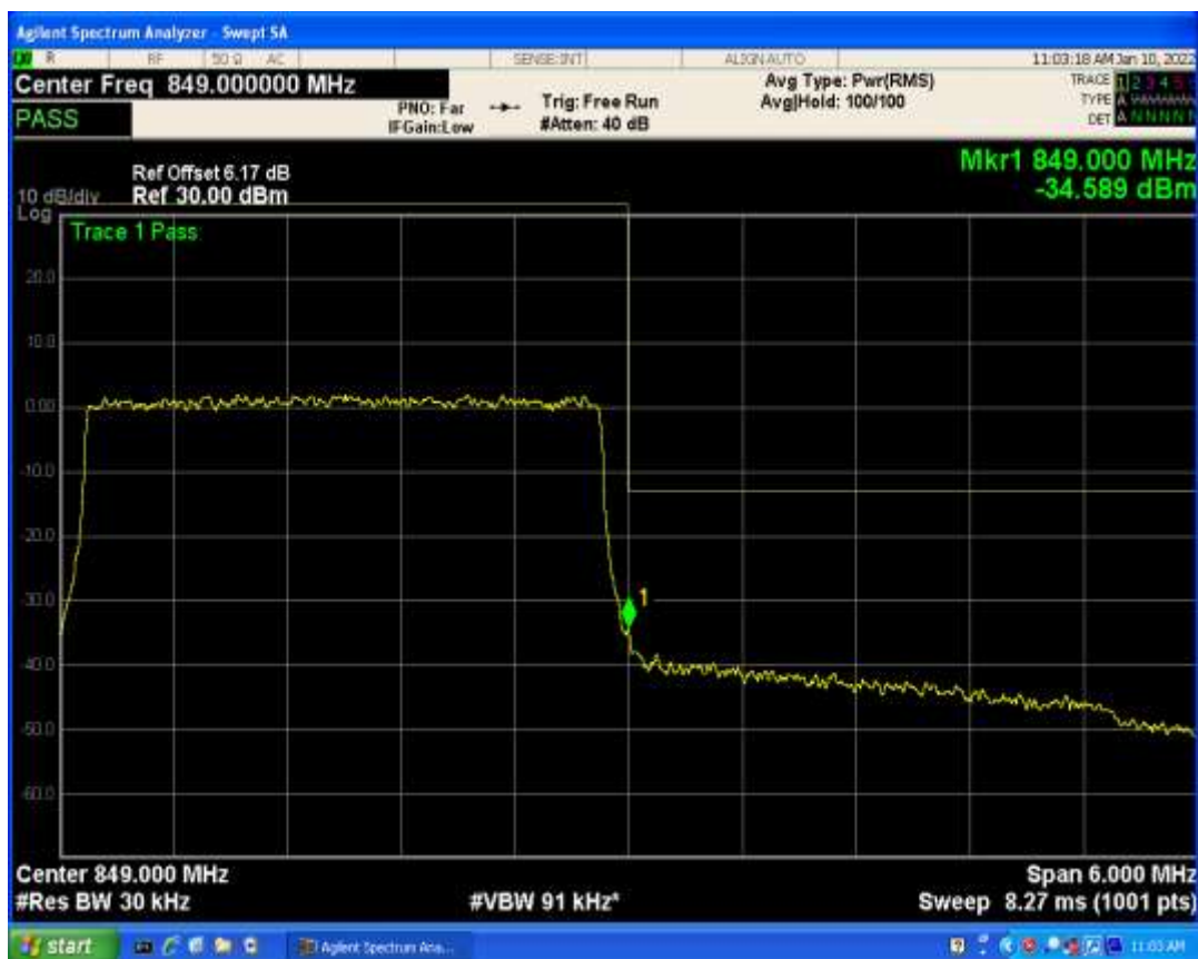
Band5 QAM16 BW=3MHz Channel=20415 RB Size=15 Position=#0
