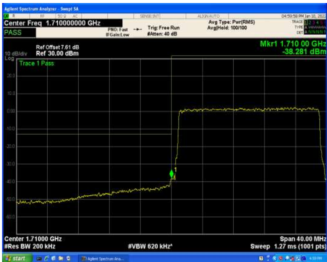
Band66 QAM16 BW=20MHz Channel=132072 RB Size=1 Position=#Max
