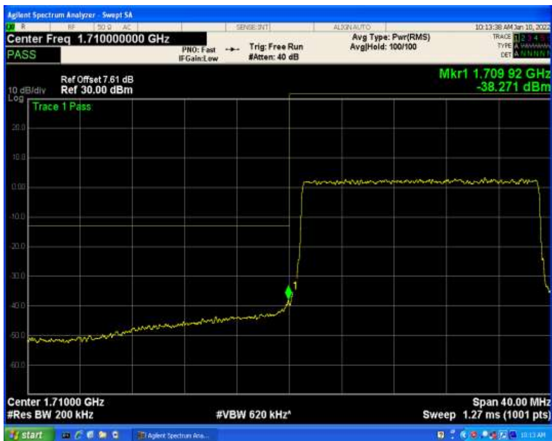
Band4 QPSK BW=5MHz Channel=20375 RB Size=1 Position=#0
