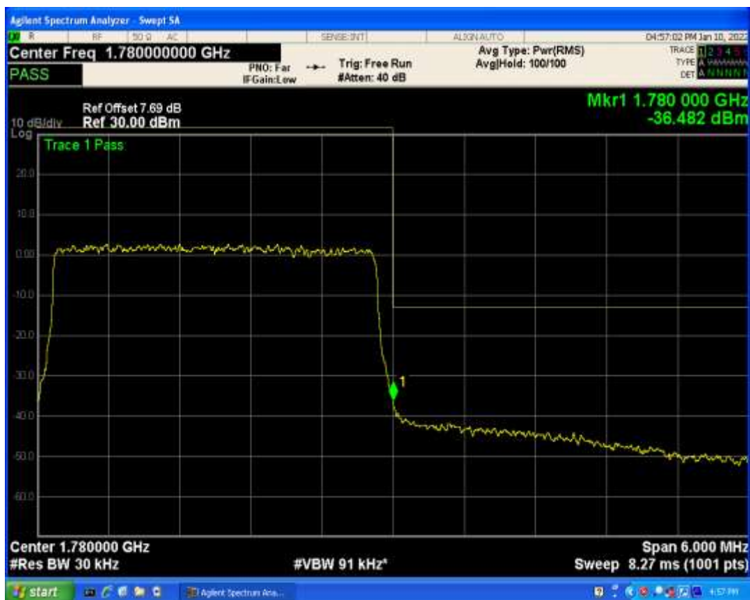
Band66 QAM16 BW=20MHz Channel=132572 RB Size=1 Position=#Max
