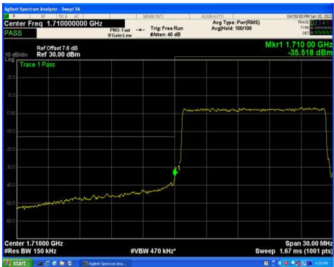
Band66 QPSK BW=10MHz Channel=132022 RB Size=1 Position=#Max
