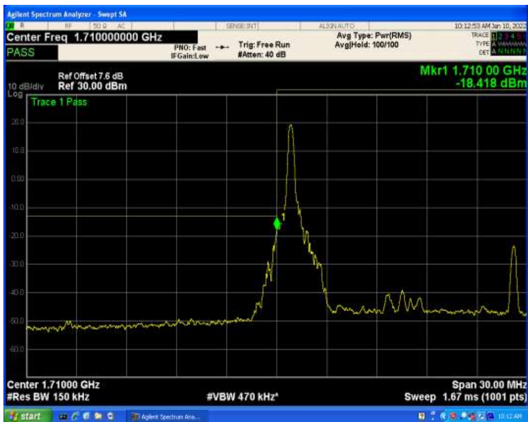
Band4 QAM16 BW=10MHz Channel=20350 RB Size=1 Position=#Max
