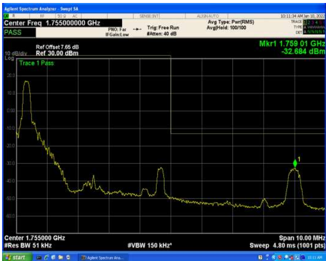
Band4 QAM16 BW=5MHz Channel=19975 RB Size=25 Position=#0
