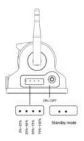
Power Button: Enter work or sleep mode for 3-second pressing, double-click to enter the standby mode, and click to enter the work mode.
