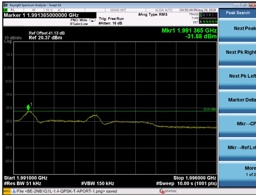
The channel power of 1MHz for 1991.365MHz is -23.63dBm, which is within the limit of -19.02dBm
