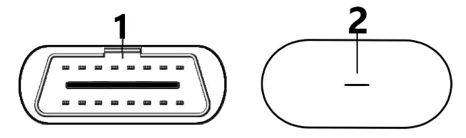
1: Vehicle Data Connector (16-pin) – connects the DFirst-201BT to the vehicle's 16-pin DLC directly.
