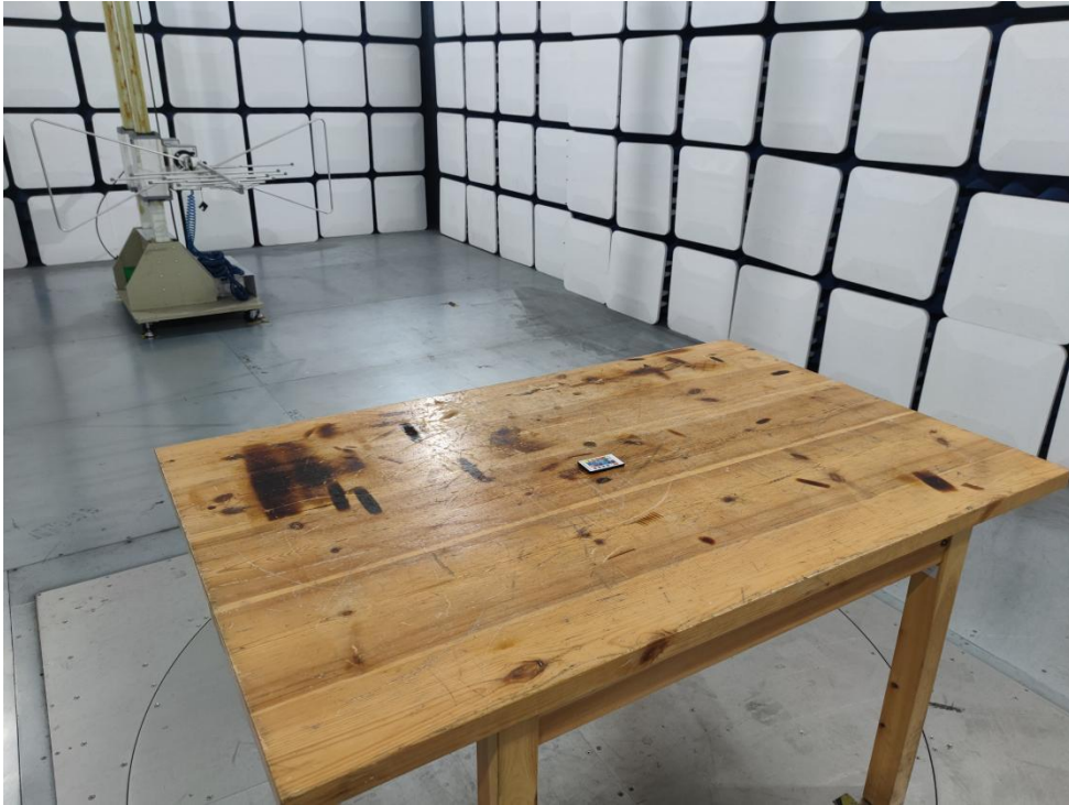
Photo of Radiation Emission Test
