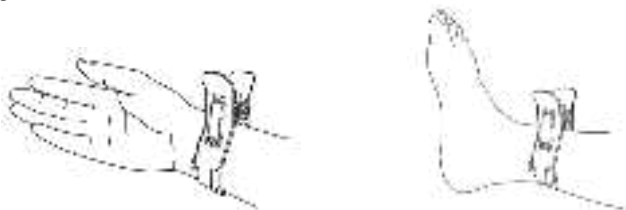
Figure 6-2 Installation of limb electrode
