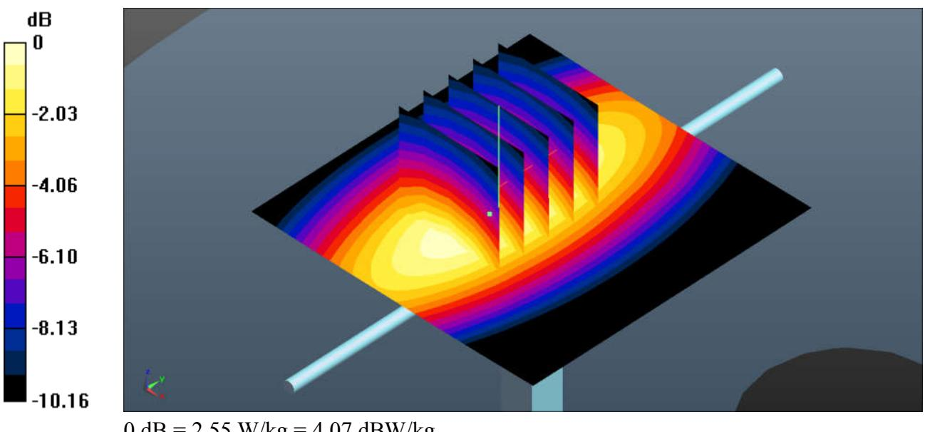
**System Check\_Head\_1900MHz****DUT: D1900V2 - SN:5d170**
