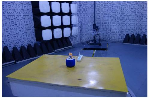
Radiated Emissions (9kHz-30MHz)
