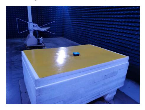
**Radiated Spurious Emissions Test View (Above 1GHz)**
