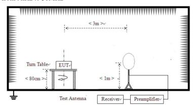
For radiated emissions from 30MHz to1GHz
