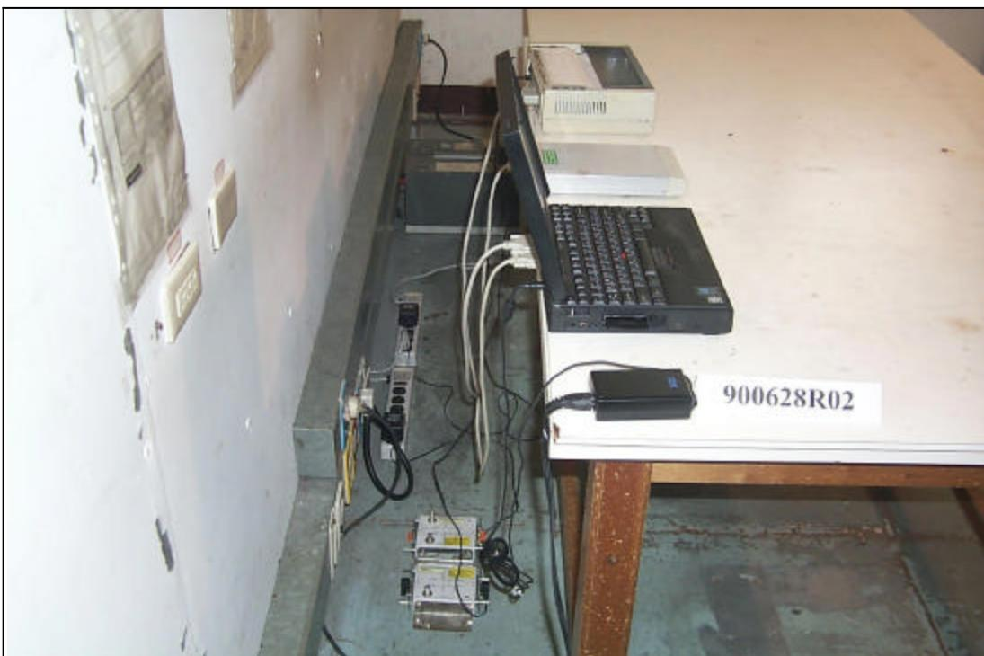
RADIATED EMISSION TEST
