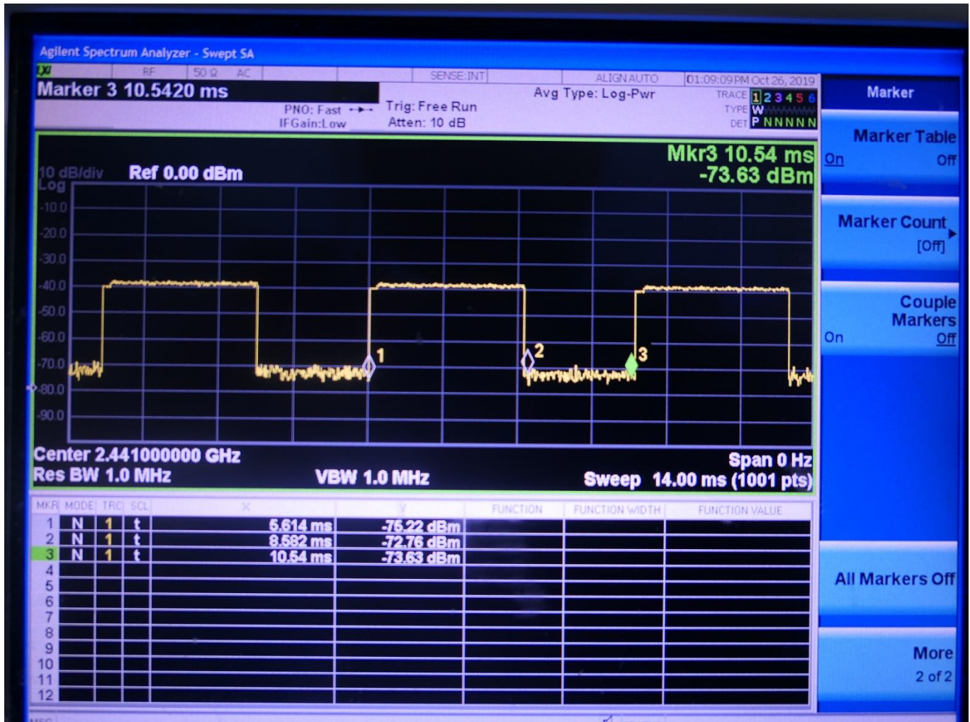
Time-domain plot for Bluetooth transmission signal
