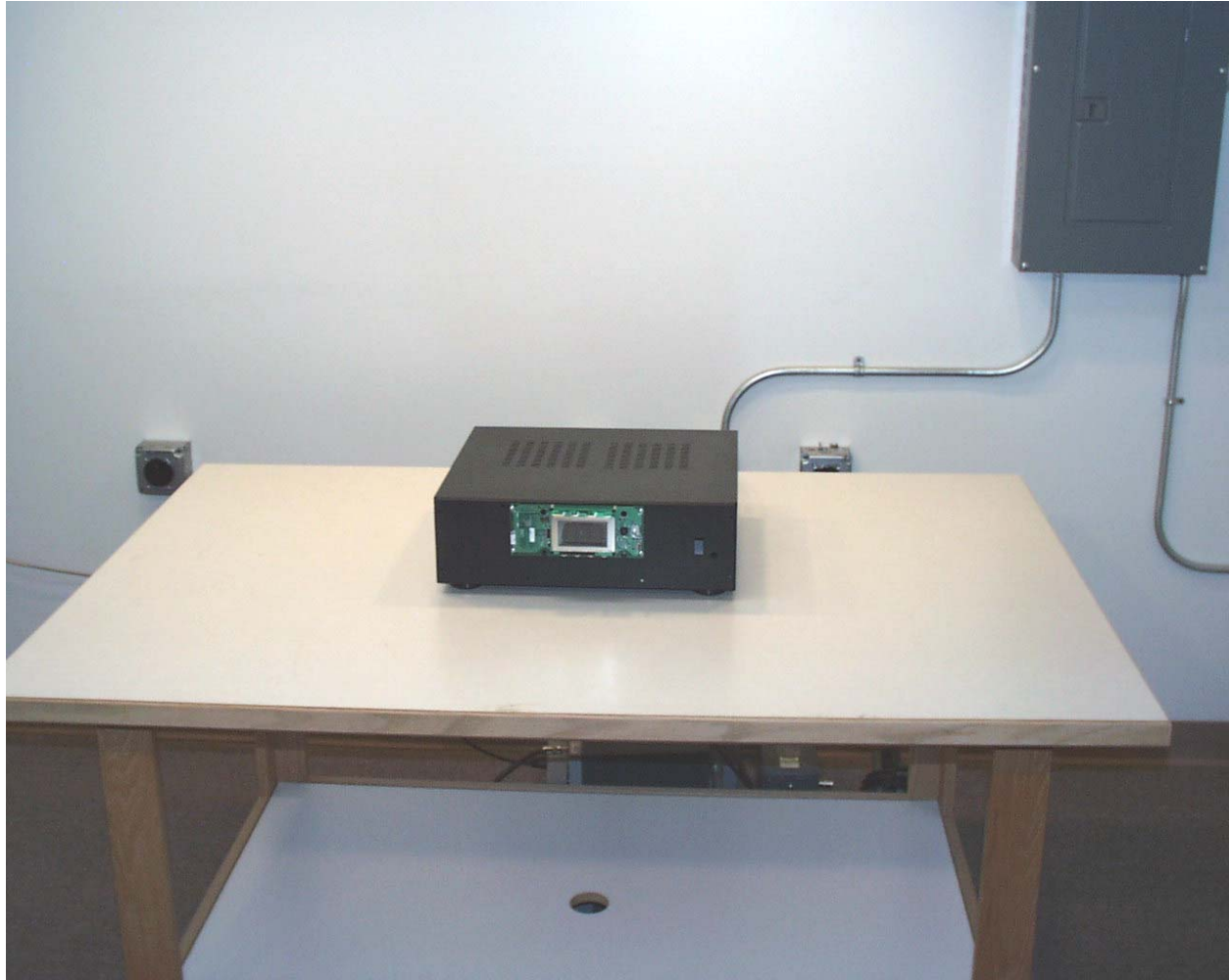
Photograph 3 - Front View Conducted Disturbance Worst Case Configuration
