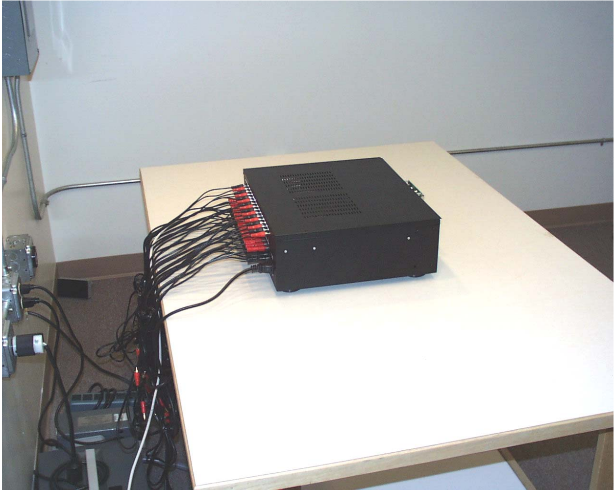
Photograph 4 - Back View Conducted Disturbance Worst Case Configuration
