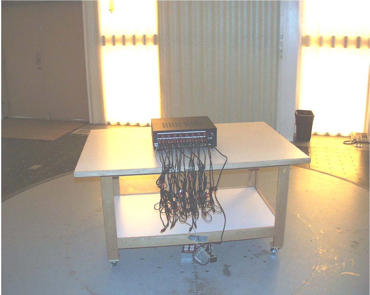
Photograph 2 - Back View Radiated Disturbance Worst Case Configuration
