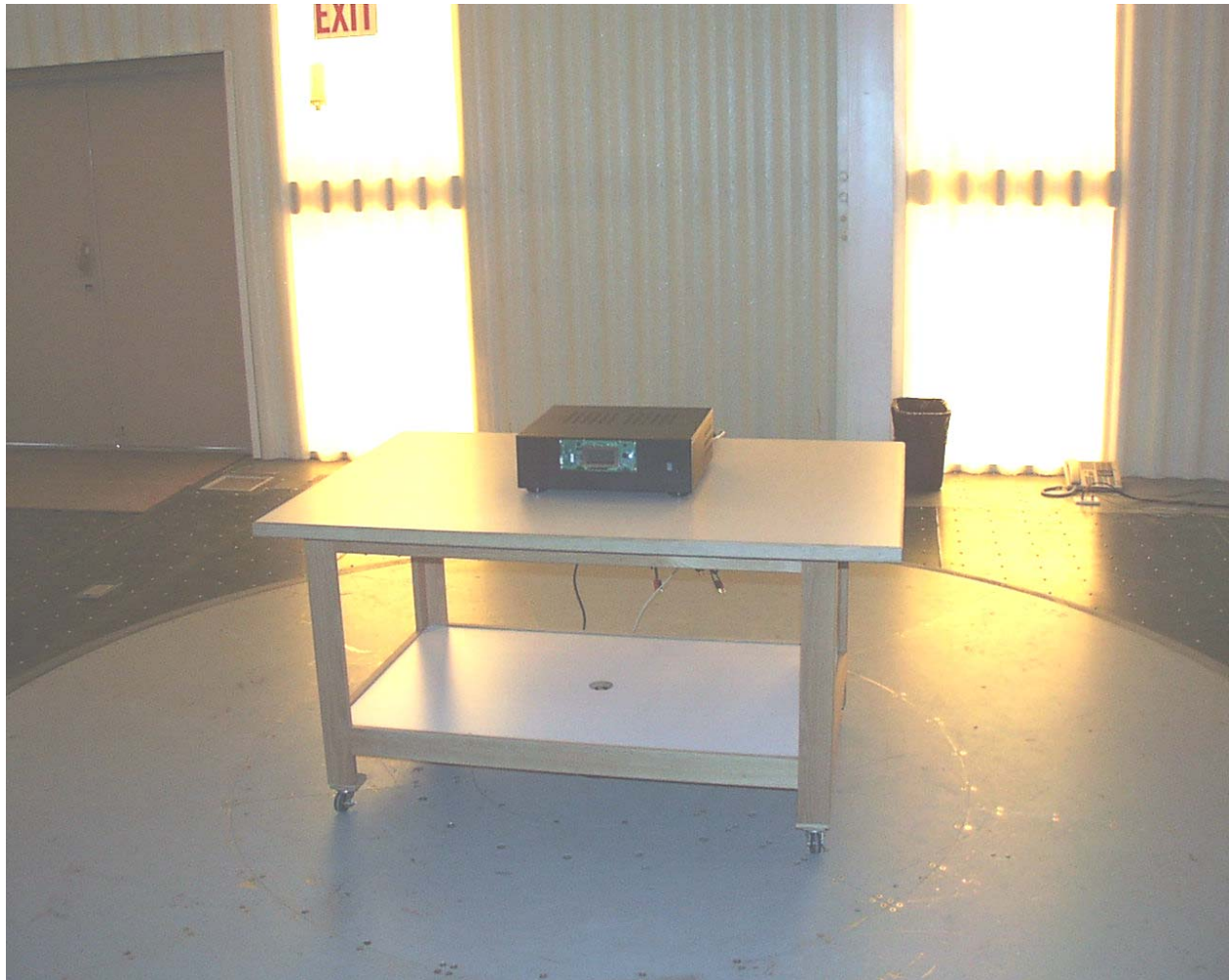
Photograph 1 - Front View Radiated Disturbance Worst Case Configuration
