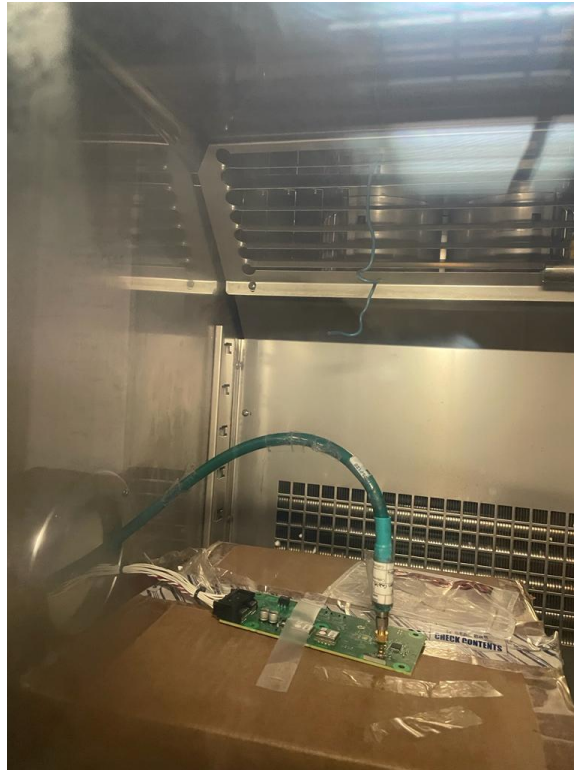
Figure B1: Conducted Frequency stability setup in Climatic chamber
