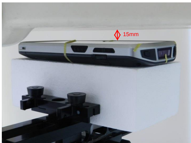
Front, Test Separation 15 mm
