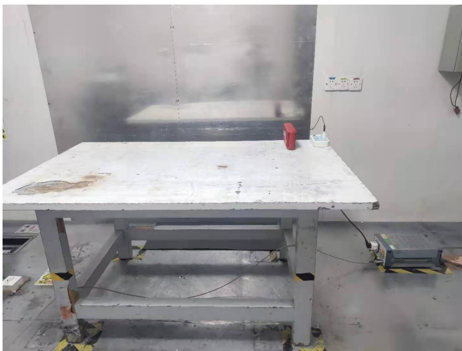
Photograph 3: Set-up for Conducted Emission on AC Mains
