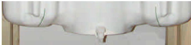
Figure 7.2 SAM Twin Phantom shell
