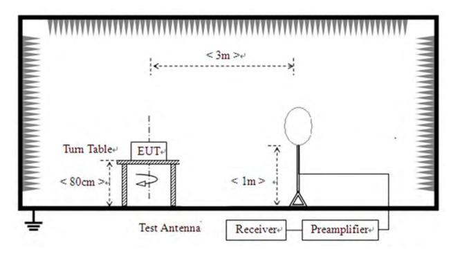
2) For radiated emissions from 30MHz to1GHz
