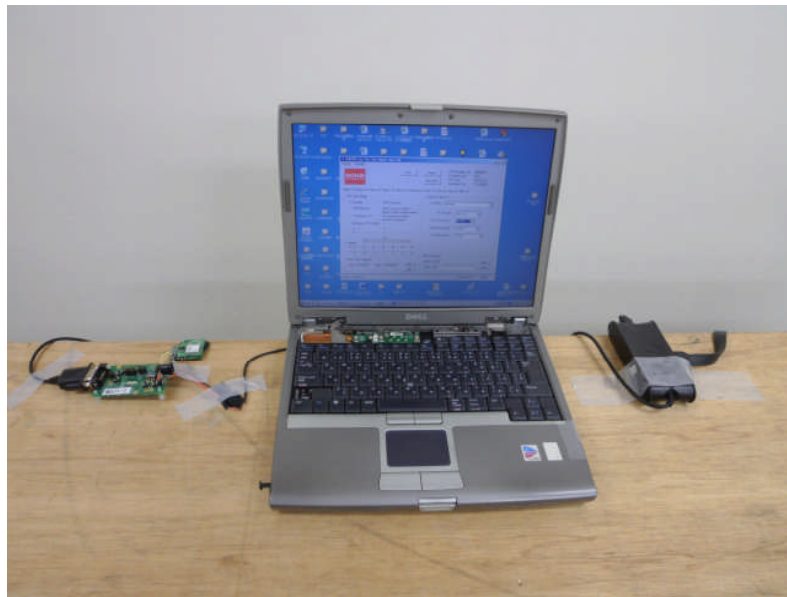
Photo5 Test setup for Line conducted(Front)
