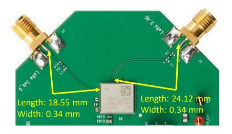
PCB for assembly the antenna
