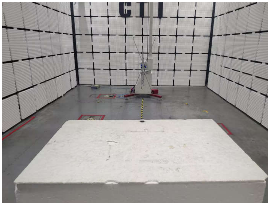
Radiated spurious emission Test Setup-1(Below 1GHz)
