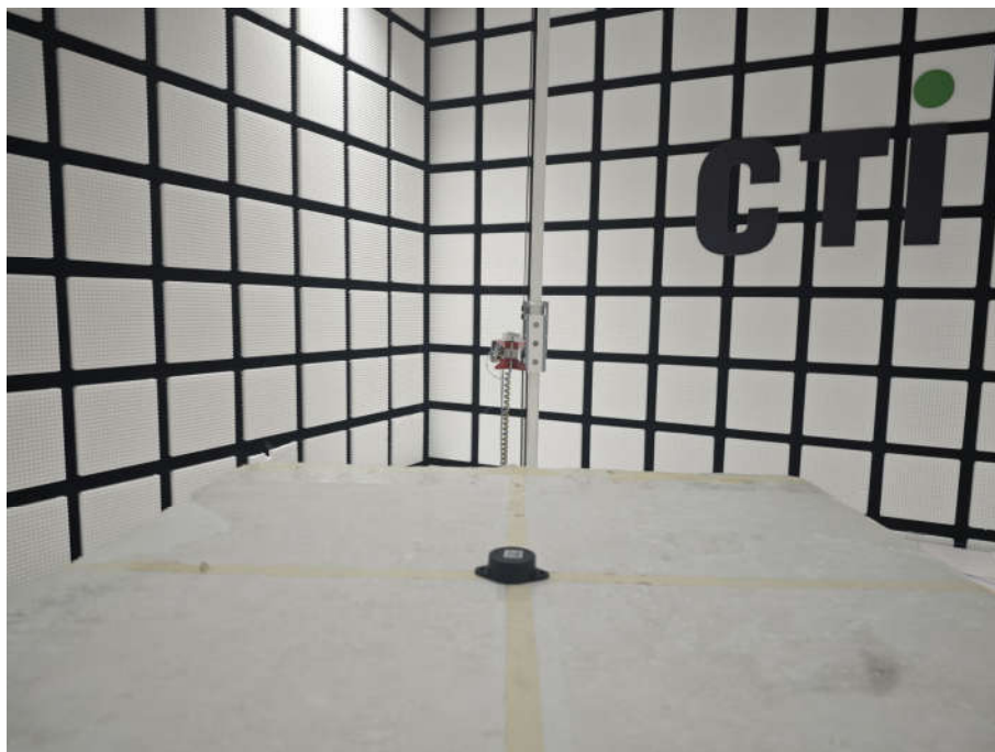
Radiated spurious emission Test Setup-3(Above 1GHz)
