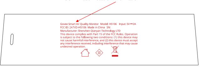
The label shown shall be permanently affixed at a conspicuous location on the device and be readily visible to the user at the time purchase (Labeling requirements per 2.925)
