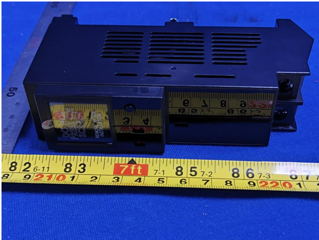
FIGURE 2 240 VAC 30 A WISER CONTROL RELAY (QO200PWX240) BACK APPEARANCE
