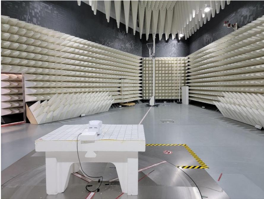
**Photograph 1: View Test Set Up Radiated Emissions 30 – 1000 MHz**
