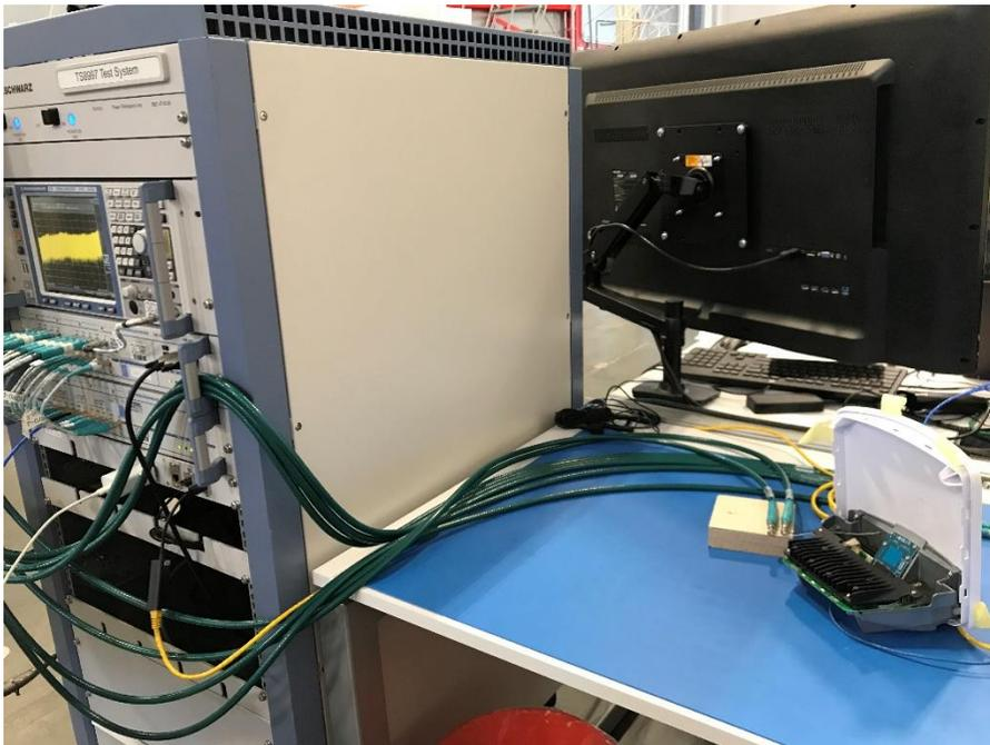
**Photograph 4: View Test Set Up RF Conducted**
