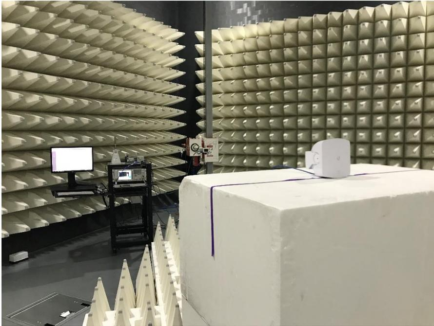
**Photograph 3: View Test Set Up Radiated Emissions 17 - 40 GHz**
