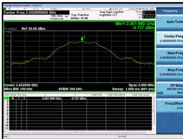
GFSK (BLE 1Mbps) LOW CHANNEL, CARRIER LEVEL
