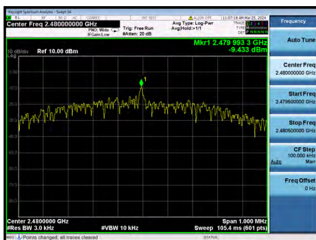
GFSK (BLE 1Mbps) HIGH CHANNEL
