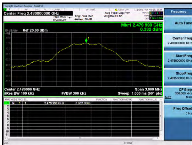
GFSK (BLE 1Mbps) HIGH CHANNEL, CARRIER LEVEL
