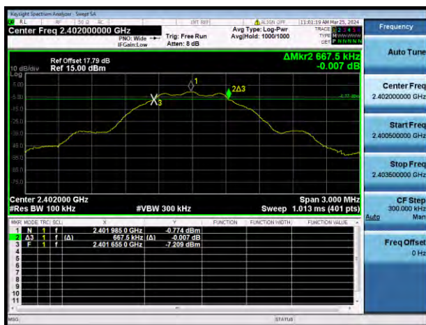
GFSK (BLE 1Mbps) LOW CHANNEL
