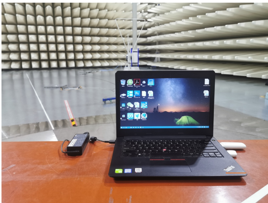
Spurious Radiated Emissions Test setup (below 1GHz)
